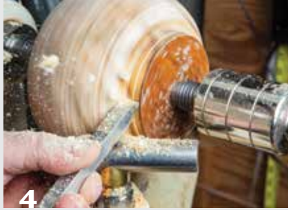
4 Beginning to form a tenon at the tailstock end of the blank.
