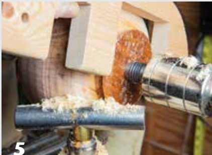
5 The author's tenon-sizing gauge, made from scrap wood, used to quickly form a tenon you know will fit in your chuck.
