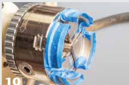
10 Painter's tape protects the wood as you gently expand the jaws inside the mortar rim for a good grip. Use the tailstock live center to aid in centering.
