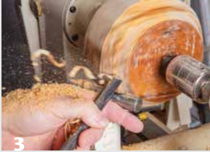
3 Rough-shaping the mortar's outside profile, cutting toward the headstock and across the facegrain. The blank is mounted between centers.
