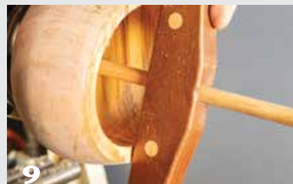
9 Deepen to desired bottom thickness, checking often with a depth gauge.
