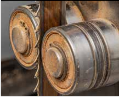
18. Guides – Position the guides so the front of the roller is just behind the tooth gullets.
