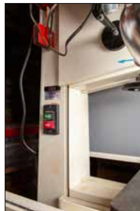
7. Steel – Large new saws tend to be fabricated from sheet steel. This makes it cheap to ship in pieces for on-site assembly.
