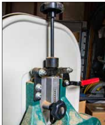
6. Heavy – Older cast-iron machines are heavy and vibrate less than modern welded-steel constructions. Note the red quick-tension-release lever on this saw.
