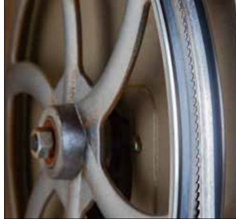
12. Gullets – The rearmost part of the gullets should ride on the peak of the tire crown. Here, the blade is too far forward on the tire.
