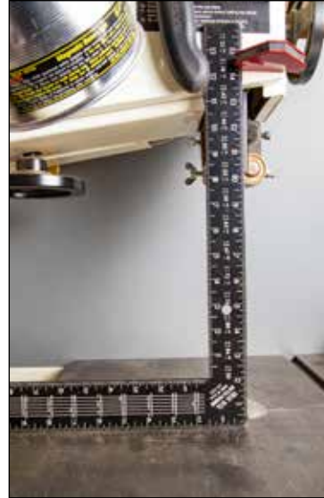
4. Tall throat – The depth of cut specification is the maximum thickness that can be cut with the blade guides fully open; on this saw, the blade tension adjustment wheel hangs low and would interfere with some cuts.
