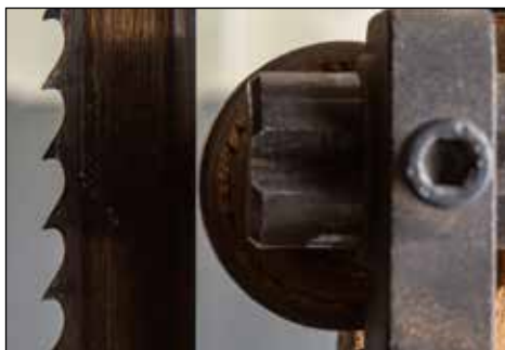
20. Clearance – The thrust bearing is adjusted to a small clearance at no power. Some use a dollar bill as a gauge, I just eyeball it.
