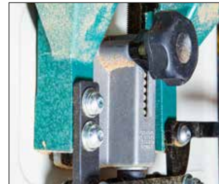
15. Another – Make small adjustments under hand power, then check at power and lock the adjuster. Here's the tracking adjustment on another common saw.
