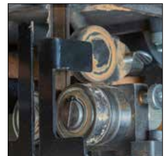
22. Lowers – Lower guides are adjusted exactly the same as the upper guides.
