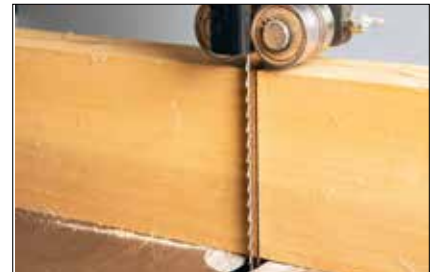
D. The back edge of the blade slides easily into the cut.
