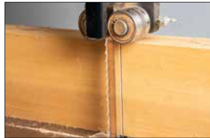
C. Leaving the saw turned off, slide the cut block around the back of the blade.
