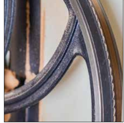
13. Crowned – This blade is adjusted about right. The back edge of the gullets rides on the crown of the tire.
