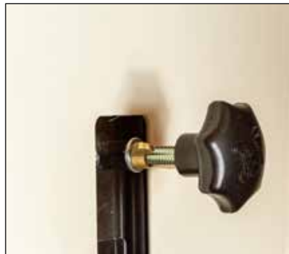
14. Adjuster – The wheel tracking adjustment knob, with locking wing nut, is located on the back side of the upper wheel cabinet.
