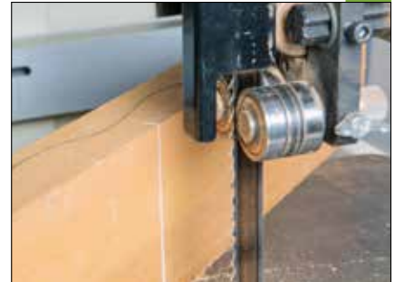
B. Turn off the saw and leave the wood standing on the surface of the table.
