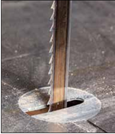
11. Teeth – When installing a blade, be certain the teeth are pointing down at the table top.
