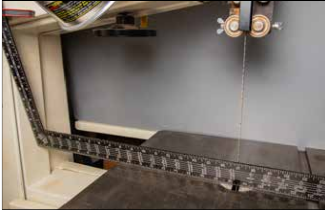
3. Wide throat – The throat specification is the largest cut possible from the blade to the frame. My 18" (45cm) saw really can cut an absolute maximum of 18-3/8"(46cm).
