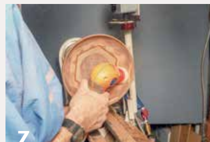
7 The interior is reshaped and the walls thinned. With the work mounted securely in the chuck, the author power-sands and fills the central hole with epoxy.
