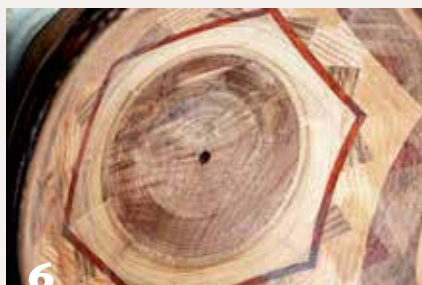
6 The author turns away the inlay in the bottom, revealing a solid Walnut block with a threaded hole. Apparently, the bowl had been mounted on a screw at one point.
