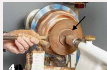
4 A chucking tenon is formed in the bottom (see arrow) for a later mounting. Also, the body of the bowl is trued and reshaped.
