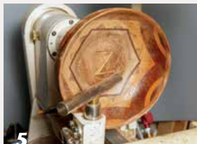
5 With the underside thinned and reshaped, the interior is addressed while there is still sufficient wall thickness for some cutting and reshaping as needed.
