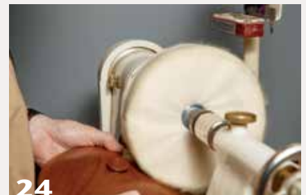
Once the finish has cured, both the lid and the bowl make a trip through the lathe-mounted buffing wheels to achieve the final sheen.
