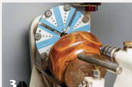
3 The author first mounts the bowl on a set of jumbo, or Cole, jaws, along with the tail center for support. Note the tape on the jaws to protect the workpiece.
