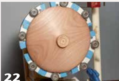
Now the lid is remounted on the jumbo jaws to provide access for turning the knob/pull.
