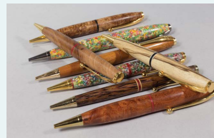
Not using the kit's centerband gives you lots of design flexibility. You can make the pen shorter and go with or without trim decorations added to the blank before turning.
