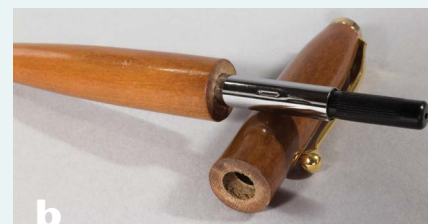
You can make up the difference in length, or not. This blank is left longer than the brass tube inside it to compensate for the missing centerband.
