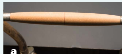
Turning blanks for a pen with no centerband means you can turn the interface fit continuously. Makes for the perfect fit.
