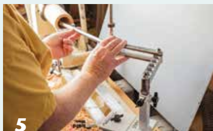
5 The author uses a deep-hollowing rig to open the inner diameter to accept the mug insert. The challenge with this hollowing task is to overcome the need to work far beyond a standard toolrest.
