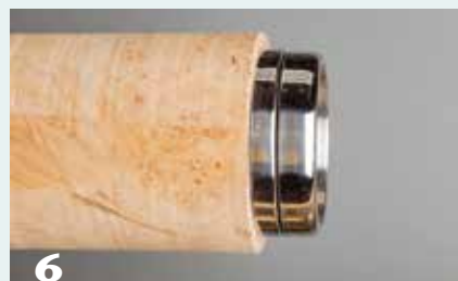
6 Work incrementally from the top-to-bottom of the blank, stopping frequently to test fit the insert.
