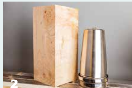
2 The blank must be long enough to accommodate faceplate or chuck mounting, room to part-off, final wall thickness, and a little more than 6" depth for the insert.
