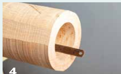
4 Measure the depth of the hollowed interior. You may need an extension for your Forstner bits that will allow you to drill just deeper than 6".
