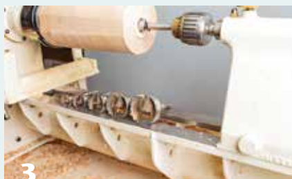
3 Remove the bulk of the waste material from the interior of the blank with a series of Forstner bits, stopping just short of the diameter of the insert.
