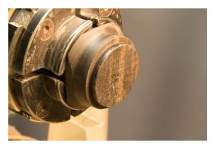
Here is the bottom of the top finial "base", the piece that will fit into the opening of the shell. There is a shoulder to rest on the top of the shell as well as a bit of an inside "plug" to help block seeing any flaws in that opening of the shell.
