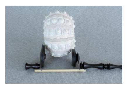
Here are all of the parts of my ornament assembly. Top finial, top finial base, shell (of any kind), bottom finial base, and bottom finial. All of the pieces that will be held together with a piece of bamboo kabob skewer. No wasted wood by turning little finials out of much larger diameter stock.
