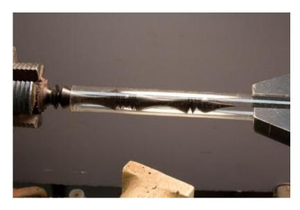
A more appropriate sized "catchers mitt" and a smaller chuck to hold it in place. There is no contact between the finial and clear tube so there is no need for the tailstock to rotate. The tube is only there to catch the finial to prevent damage when parted off.
