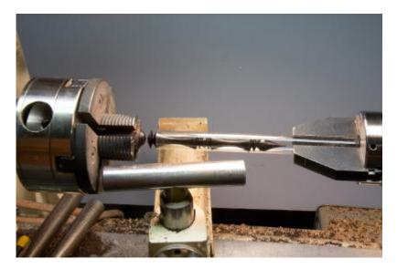
This is a pretty simple yet very powerful concept. A simple plastic tube, cup or any vessel that can be held, placed so it surrounds the work as it is parted off frees your hands and your mind. Using this and the toothpick (or anything else) in a drill chuck to catch any piece with a hole when parting off has many applications in turning.
