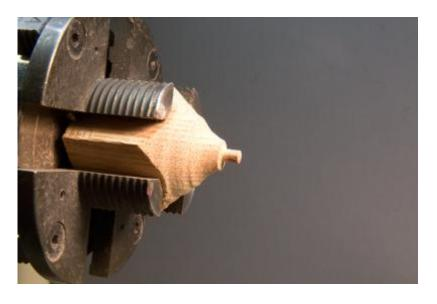
Custom turning mandrels as needed is a worthwhile skill to develop. Here a scrap piece of oak is used to make a mandrel for the finish turning of the upper finial. The finial was already drilled for the kabob diameter and that hole is used for the mounting on the mandrel.
