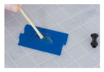
With the ends crushed, why not use the kabob skewer as my mixing stick? Saves getting something else dirty and helps work the adhesive into all of the fibers on the crushed end of the skewer.
