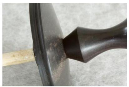
This interface is a surface to surface mate. Both surfaces should be clean and flat so the seam is not noticed. A small bit of pressure on the joint while it is setting up isn't a bad idea to keep them in intimate contact.
