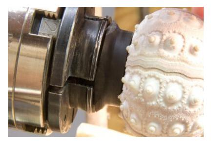
The top finial base seating is a trial and error fit for diameter and spike clearance. Tuned until I'm happy with the fit and seating. There is a very small amount of clearance intentionally allowed between the shell and wood diameters.
