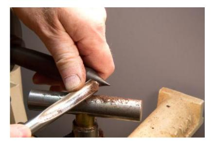
A more effective way to cut delicate spindles, mounted only from one end or between centers, is to support the cut with your own "spindle steady". If you "squeeze" the work between the cutting edge and your spindle steady, there is no reason for it to flex. It only rotates between the two equal and opposing forces.
