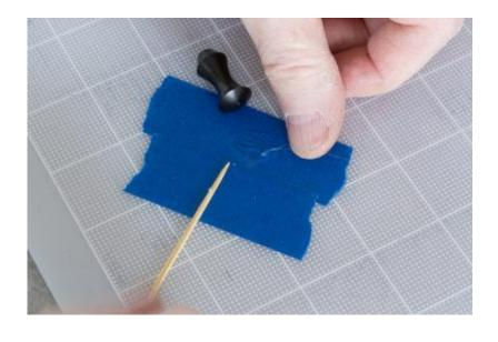
I use epoxy for all of my fastening needs on ornaments. I like the open time, the ability to fill gaps, and the long-term flexibility of the material. The hole has been wetted with glue and here the knot is coated with glue as well.
