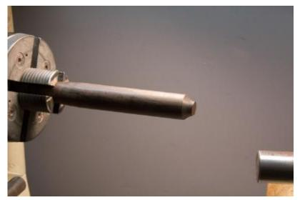
Not only does the work flex away and chatter, you usually will wind up with spirals to go along with your design. As you get closer to the headstock, it is less of a problem. BTW – the other end of the finial has already been drilled with the kabob diameter hole.
