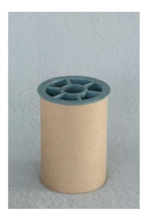
Another high tech assembly fixture. A cardboard core from a copier paper roll. I cut them down and use them for ornament shipping containers. Here is a short cutoff length with the spindle core in place. The shaft hole becomes a perfect positioning device for positioning the ornament for gluing and to let is rest until cured.
