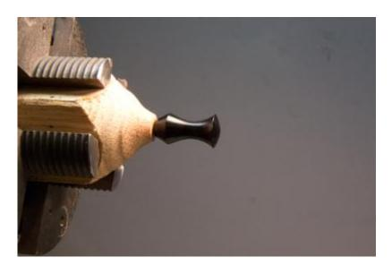
Turned, sanded, and finished. When running on a stub of a mandrel like this, sharp tools and light touch are the keys. These are good skills to develop regardless of your turning interests. At this point, time for a quick center drill and then drilling for hanging line.
