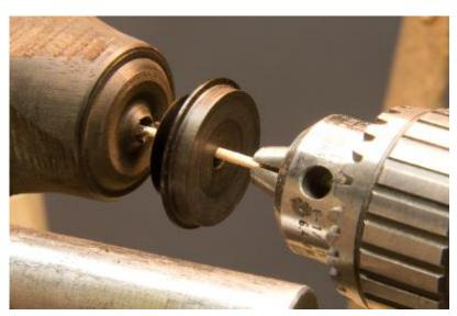
Top and bottom finial "bases" are turned as much as possible when mounted in the chuck. Then are parted off and reverse mounted in the chuck for completion on that side. The small inner diameter on each can be marred in work holding as they are internal. Here a toothpick is used to capture the bottom plug on separation.
