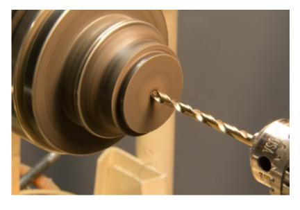
I use a piece of bamboo kabob skewer to hold my many ornament component pieces together. Here is the drilling to pass the kabob skewer through. The diameter is drilled to be a slip fit to allow for gluing.
