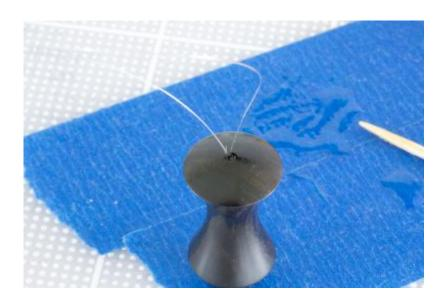
I try to get sufficient glue in the hole so that it fills. I'd like to see it at or close to the top of the hole. Not so much for strength but for appearances. Any open depth showing at the top of the hole is visually distracting if someone examines things up close.
