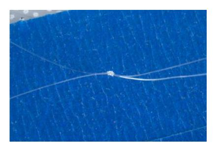
With the previously drilled finial hole sized large enough for my 2# test line knot, I cut off a length of line. After determining the desired loop size, I tie a knot to help secure it in the hole when glued.
