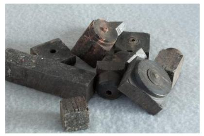
With Blackwood currently costing over \$10/lb, I hesitate to use larger diameters and cut away most of it. I make the finials as assemblies. Each of the respective pieces made from various sizes of stock to minimize wastage. I do try to match colors and grain.
