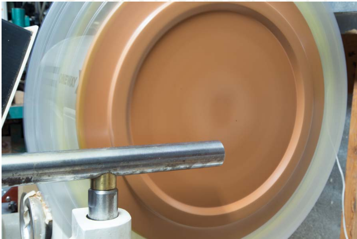
Figure #12: I had to move the bumpers in a bit and mount the biggest piece of platter work that I had. As expected, they ran true, held well, and worked flawlessly.
