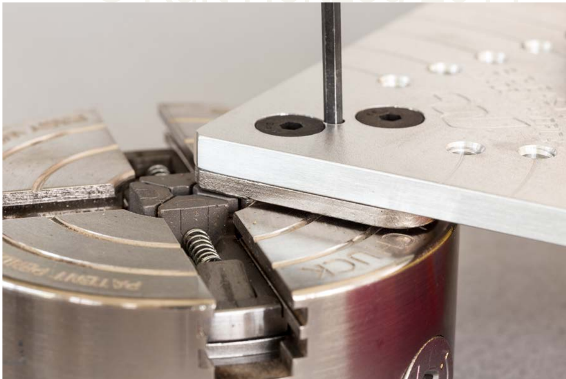
Figure #8: A simple push through the hole and the jaw is released. All of the jaws are location interchangeable with no special positions required.
