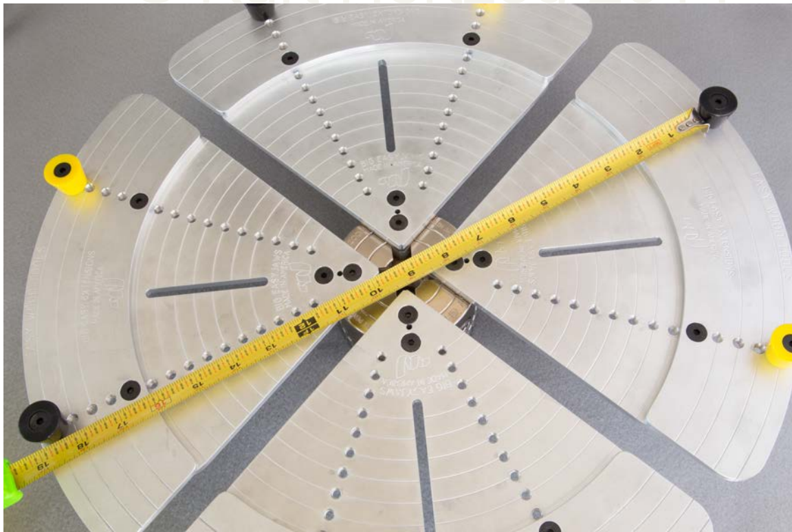
Figure #10: The Big Easy Jaws with the Big Easy Jaw Extensions installed gives 18" compression style grip size. In an expansion mode, they hold 19 1/2".
