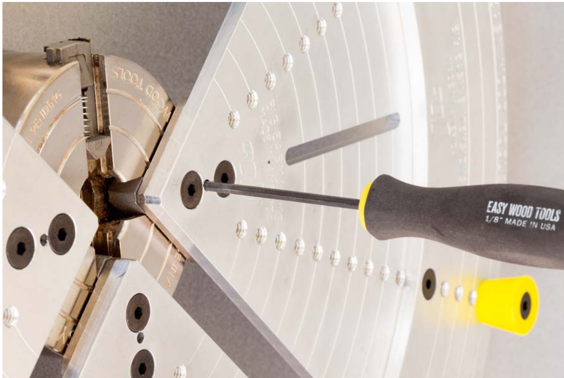
Figure #7: Although the access hole for jaw release is on the front of the jaws as opposed to the underside, they are just as easy and quick to release.
