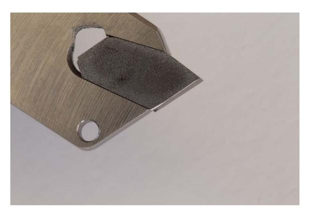
Figure #17: The replacement cutter is positioned in the tool as shown. No force is needed to get it to the proper position for seating with the EWT Flex Key as it easily slides into place.
