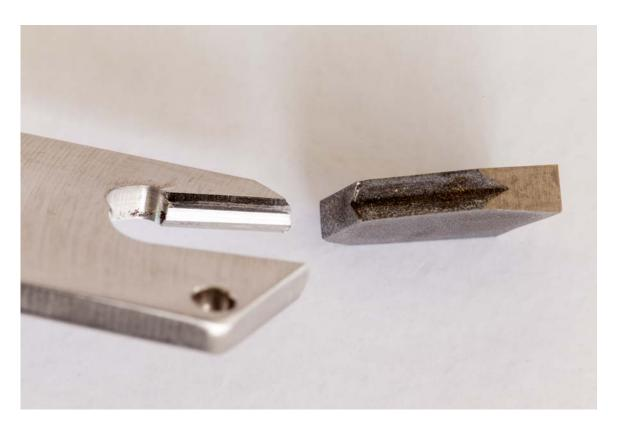
Figure #21: There is a mating V milled into the top of the tool that will lock into the V on the carbide cutter.
