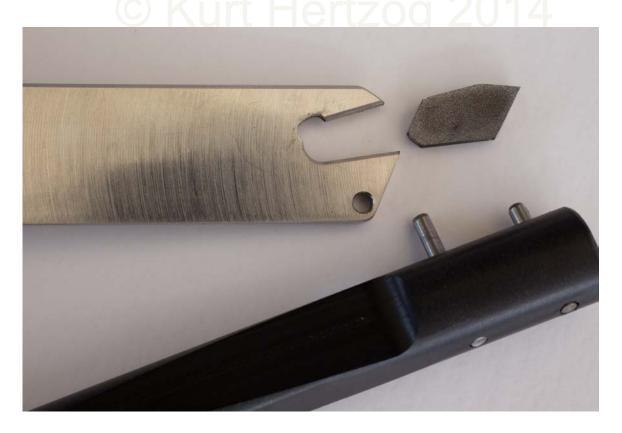
Figure #16: The unlocked carbide cutter is now removed by hand. It can now be swapped for a replacement cutter or touched up with a diamond hone if you desire.
