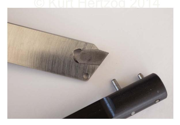
Figure #10: Its use shown very well in their instructions, the EWT Flex Key has one post longer than the other. The longer post is placed in the hole in the tool below the carbide cutter.
