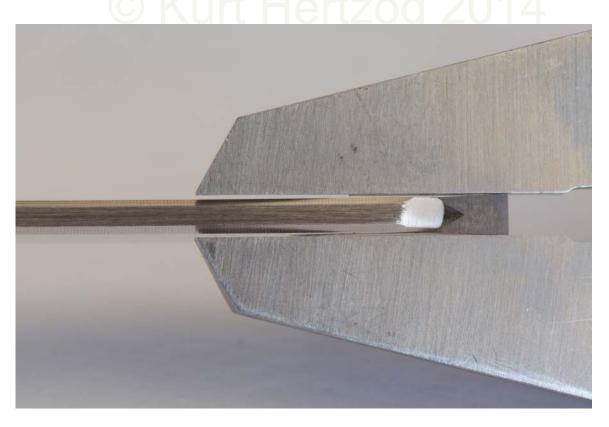
Figure #8: The tool mirrors this thinned tool thickness being just proud of 0.100". With the first  $2 \frac{1}{2}$ " of the tool having of this thinned wall, it can fit into just about anywhere.
