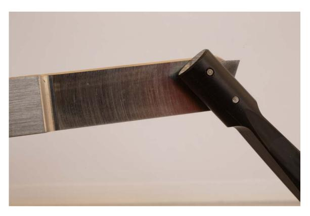
Figure #11: The shorter post is placed in the opening just behind the cutter. A very easy movement of the EWT Flex Key frees the carbide cutter allowing for replacement.
