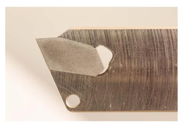
Figure #19: A small rotation of the EWT Flex Key around the long post in the hole on the tool seats the carbide cutter into the proper locked position indicated by flush on the front face.
