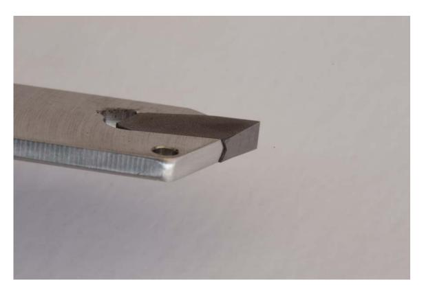
Figure #15: The amount of protrusion is indeed very small yet that is all that is needed to free the cutter from its seated ready for use position.
