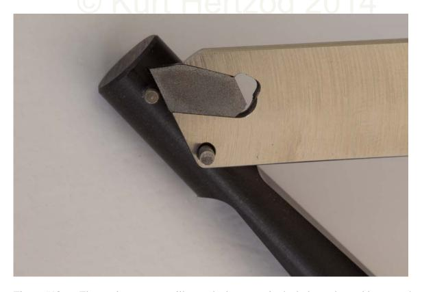
Figure #18: The seating process still uses the long post in the hole on the tool but now the short post is positioned on the front face of the carbide cutter.
