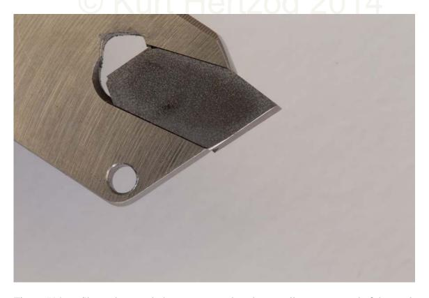
Figure #14: Shown loosened, the cutter extends only a small amount proud of the steel tool face. Being "unlocked" at that point, it is ready for changing.
