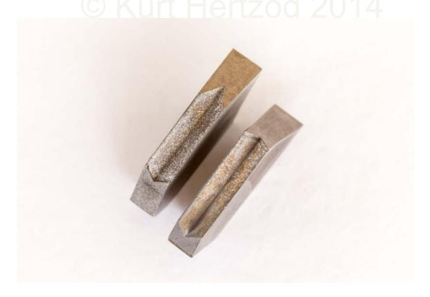
Figure #20: The trick to getting the carbide cutter to lock into place is the brilliant locking notch system in the tool. The carbide cutter has a V notch molded into the top and bottom.
