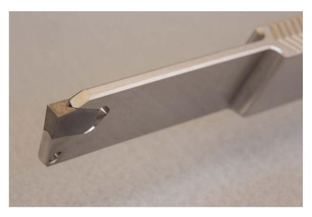
Figure #3: The business end of things is the 6" of tool extending from the 20" overall length with the 1/8" wide carbide cutter on the end.
