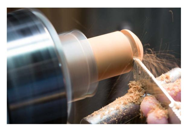
Figure #5: Even though the wider cutter face cuts a small clearance to minimize friction and heat generation, good practice is to "stair step" your cut.
