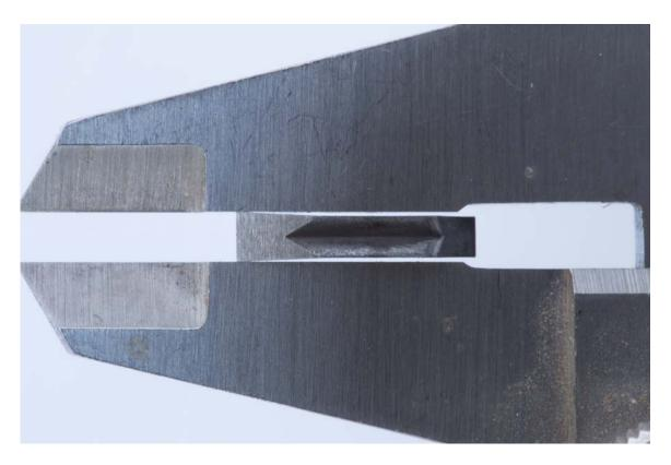
Figure #7: Cleverly designed to cut its own clearance, the front face of the cutter is 0.125" while it necks down to a shade over 0.100".
