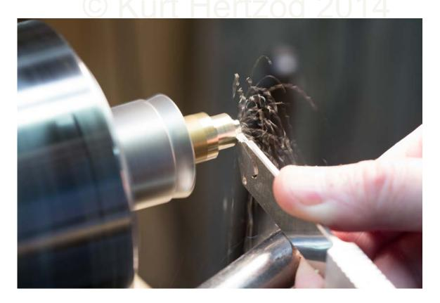
Figure #6: The full length handle allows for better control and the carbide cutter makes this parting tool ideal for materials in addition to wood. It works nicely on soft metals as well.
