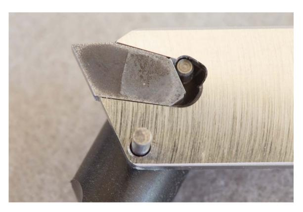
Figure #13: A slight rotation of the EWT Flex Key moves the cutter forward unlocking it for removal. The short rod will hit the stop position to prevent launching the cutter.
