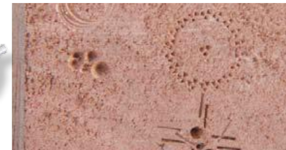
ABOVE: The finer resolution in repositioning without the pin in the tailcentre (left top) vs with the pin (left bottom). Similar advantage with the steb drive centre (right top) vs the standard four-spur (right bottom)
