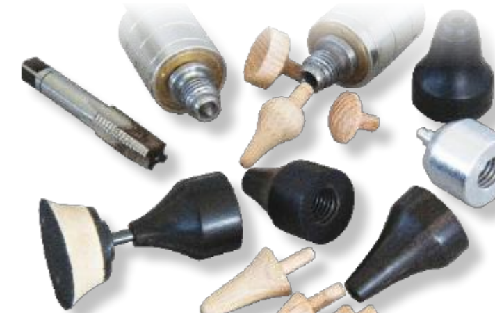
ABOVE: This tailcentre's threaded nose and knock out pin offer tremendous flexibility in making custom tapers, forms, bushings, and shafted accessory holders
