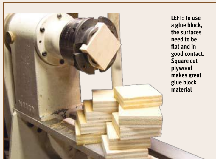
LEFT: Bonding small pieces of pricey or difficult to hold pieces of wood to a sacrificial glue block allows for the full utilisation of the small or expensive materials
