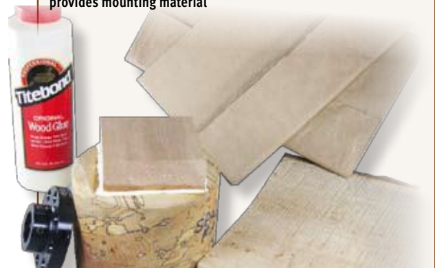
BELOW: When material thickness or amount prevents other mounting methods, a glue block with a kraft paper separator provides mounting material
