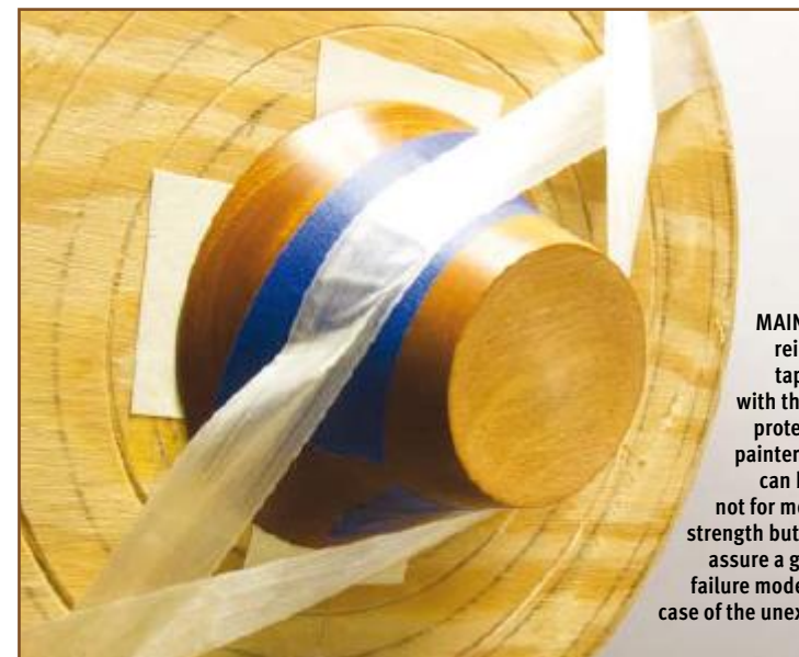
MAIN: Larger parts with more mass and perhaps more work being performed require a thicker, reinforced fabric speciality turning tape
