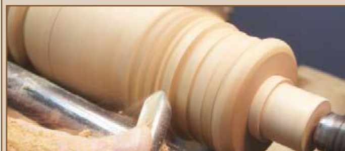
ABOVE: The stub mandrel does double duty allowing for support for turning just the lower portion without stressing the hole dimension
