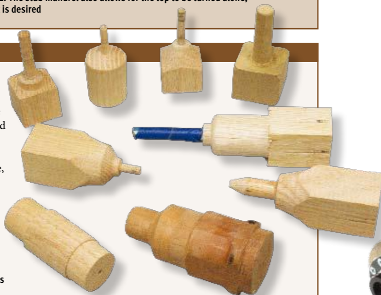
MAIN: There is no rule that says you can't make tapered mandrels to assist with the tailstock end of things
