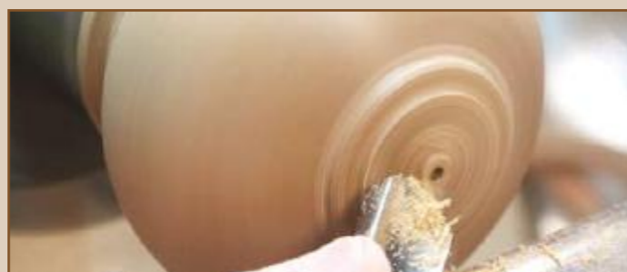
ABOVE: The stub mandrel also allows for the top to be turned alone, if that is desired
