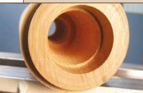
ABOVE: With the inside drillings of pepper mills stepped and identical within the family, they lend themselves to a mandrel's benefits
