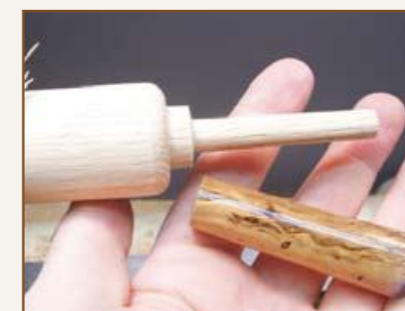
ABOVE: Closed end mandrels can be made in any size and shape to suit the needs of the part. The tailcentre can be used for additional strength, if needed
