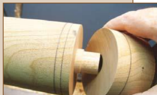
ABOVE: Using a stub mandrel to join top and bottom allows both to be turned together, if desired
