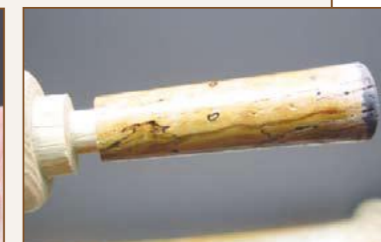
ABOVE: A light duty closed end mandrel is made and used only to re-sand and finish a closed end pen cap that experienced an ink leak
