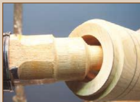
ABOVE: Support well up inside allows for turning, sanding, and finishing both with and later without the tailstock in play
