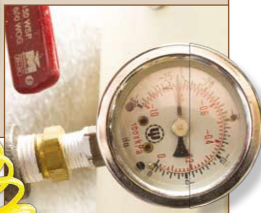
BELOW: Knowing the numbers isn't as important as regulating the vacuum applied to provide as much clamping force as possible without damaging the work
