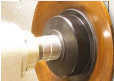
ABOVE: Vacuum chucking is as simple as evacuating the air on one side of the work and letting our atmospheric pressure push to hold the work in place on the chuck
