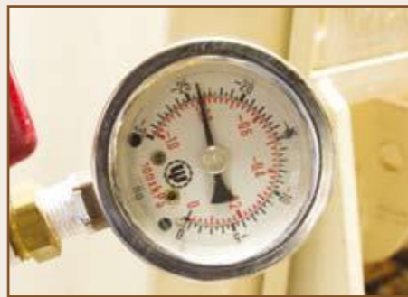
ABOVE: Full vacuum – 100kPa or 29inHg – will produce a clamp force of 14.7psi. Proportionally less vacuum yields proportionally less clamping force from the atmospheric pressure
