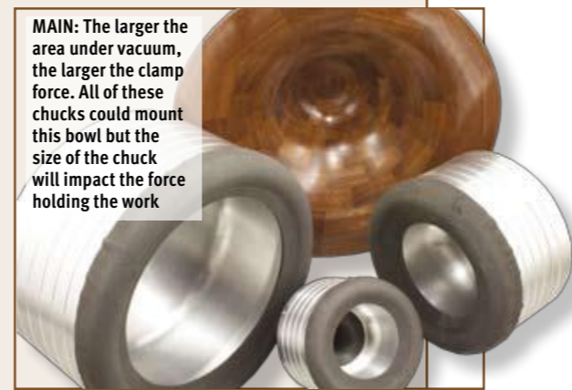
ABOVE: Full vacuum – 100kPa or 29inHg – will produce a clamp force of 14.7psi. Proportionally less vacuum yields proportionally less clamping force from the atmospheric pressure
