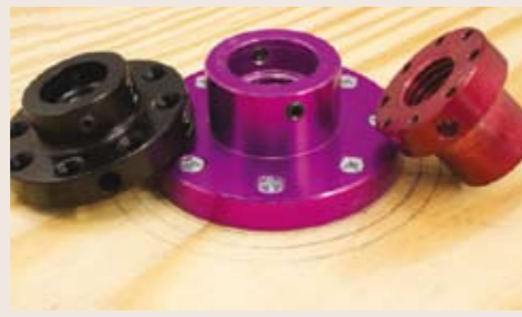
Not only prettier than the painted or rusted faceplates, the machined and anodised aluminum versions are very strong for their weight and size
