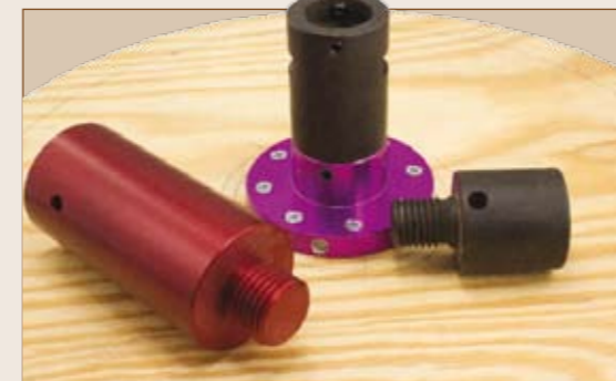
ABOVE: I try to avoid using long spindle extensions or size adaptors. I would much rather have the faceplate close to the headstock and threaded to match than extended or adapted
