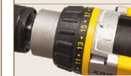
Take advantage of the gear reduction in your driver and the adjustable clutch to drive the screws home without stripping out the screws, breaking them, or damaging the driver slot
