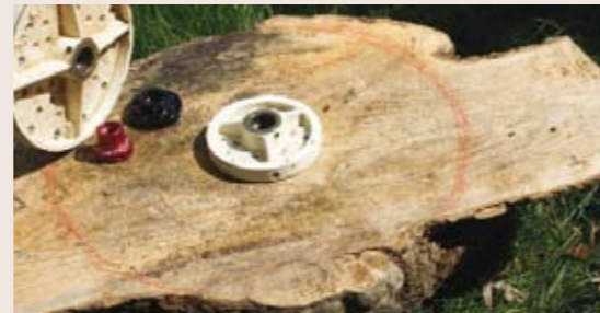
If you need a chain fall to lift your blank on to the lathe, heavy duty faceplates are in order. As shown would work but the larger cast faceplate shown on edge would be the even safer choice
