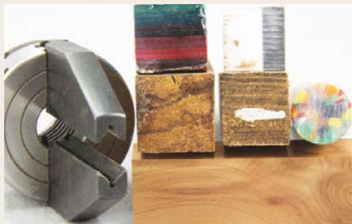
Even bent blanks can be drilled when corner clamped. There will be a material centre presented that can be drilled using the lathe. No quill travel issues here
