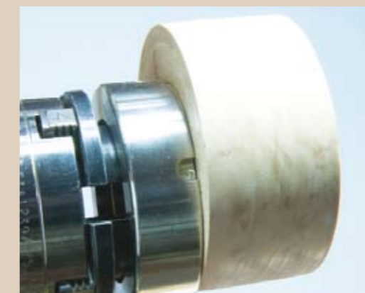
After truing on dead centre, the chuck is adjusted to the 16mm (5/8in) offcentre position for the next portion of the turning. There are precise positioning features for each position
