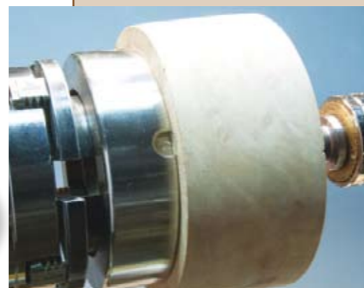
The 'o' marking indicates that it is on true centre. Depending on your design, you can use any or all of the other eight offcentre positions available
