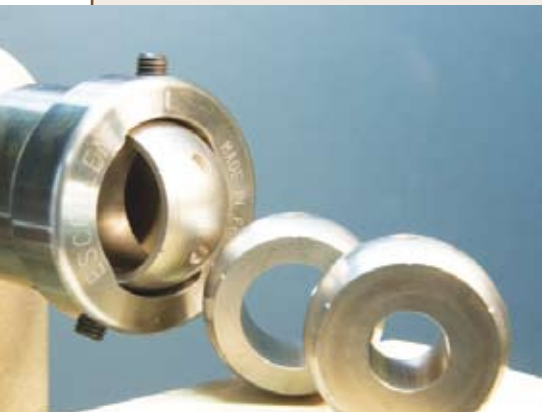
There are three different diameter tapers for you to mount your work in my Escoulen chuck. They are held totally captive by design with the amount of eccentricity locked by grub screws
