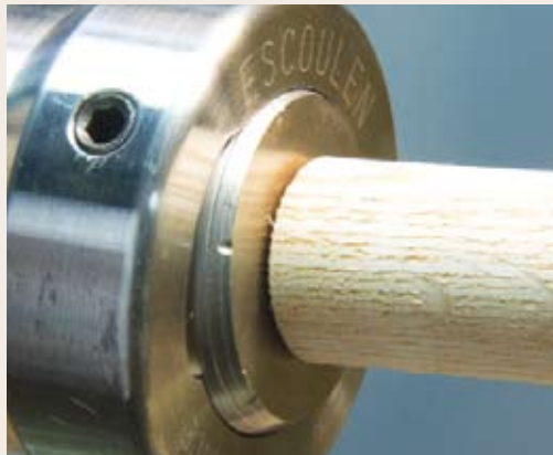
With the work pounded into the taper, the amount of eccentricity is denoted by the number and amount of rings difference between sides. There is both a pivot point screw and lock screw to fasten adjustment
