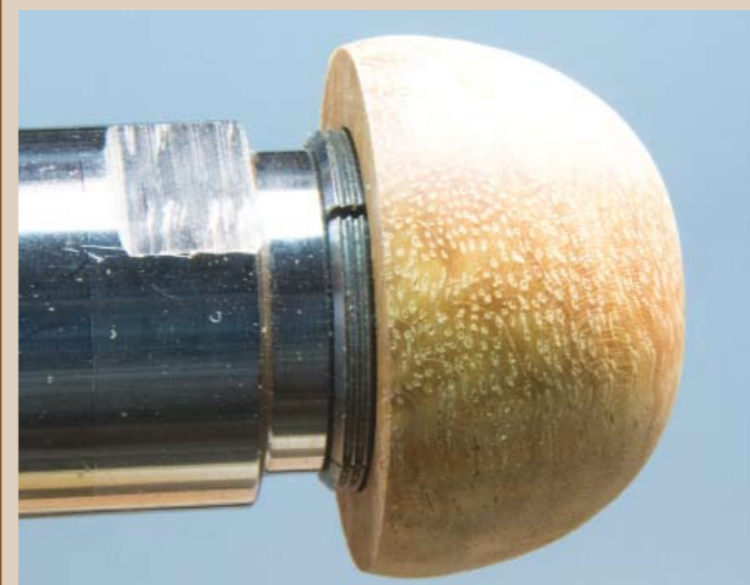
With the face prepped as flat stock, the clock chuck allows great access around the clock body for turning, sanding, and finishing
