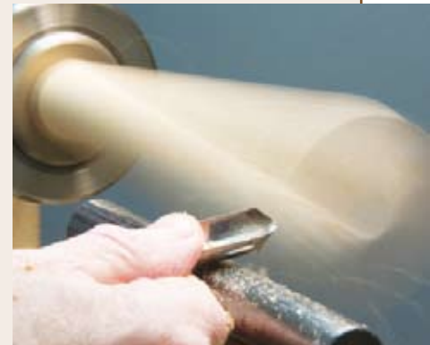
The length of your material interacts with the amount of angle adjusted in the chuck creating your eccentricity. Turning to a shadow line is an interesting experience for those new to it
