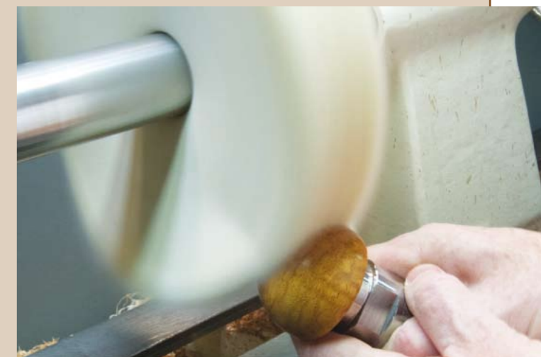
Workholding isn't just on the lathe. After turning decoration and finishing often require workholding. This chuck works very nicely to hold the clock body while buffing
