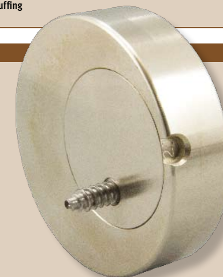
My multi-centre chuck is fastened to the lathe by expanding the jaws of another chuck into the pocket on the back. It then has dead centre and then eight different off-centre selections
