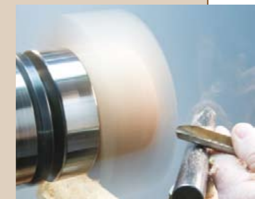
Working with offcentre turning takes a bit of getting used to. The shadow line of the material extremes is where you are typically working with the solid lines showing the constant material area
