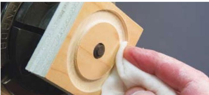
If you make a mistake and over cut, leave the mistake there. It will help you when making your next attempt. If you do need to remove it for access, do so after you have achieved the proper fit
