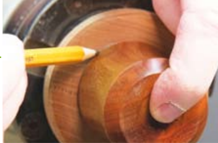
Transferring the size to ballpark the jam chuck cut can be measured but is far easier to roughly position the work and pencil mark the outside dimension
