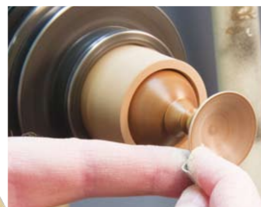
Once the tailcentre needs to be removed to provide access, lighter touches are in order whether cutting or sanding. Notice the backup support for the sanding reducing strain on the jam fit
