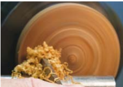
The tool of choice for cutting jam chucks is an 3mm parting tool. Ground straight across it works well for flat bottoms and walls that are perpendicular to the axis of rotation
