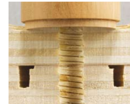
Whether a shallow inside contact or a deeper inside contact, the cutaway show the importance of the flat registration surface and perpendicular wall
