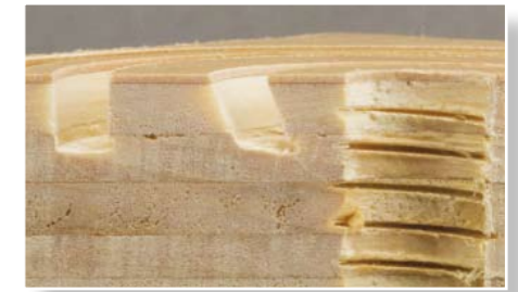
The cutaway shows the different cuts and the perils of those other than flat bottomed and perpendicular to the axis of rotation. The angled do have limited special uses
