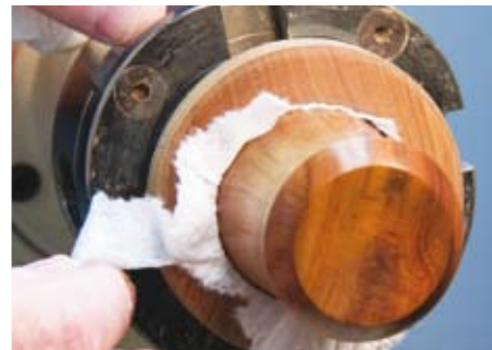
Minor over cutting can be corrected with a fold or two of paper towel or other compressible 'wood' product. If it requires too much filler, a safer alternative is to re-cut the jam chuck
