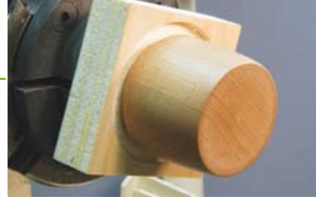
No need to clear the material outside of the immediate area of the turning. A quick and simple, cut to fit inside bearing jam chuck. Effective even with thin walls since only light sanding is planned
