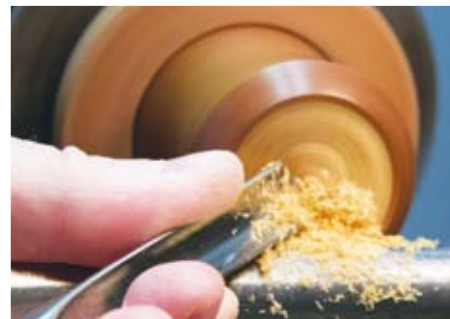
Trial and error method is used to zero in on the proper fit. Even with light cutting planned, a jam chuck with outside engagement allowing a tighter fit is used
