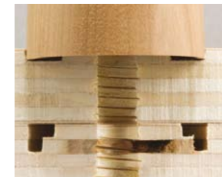
The cutaways show a shallow and a deep engagement with outside bearing jam chuck is far less dependent on wall thickness and strength. The turnings' outside circumference is incredibly strong
