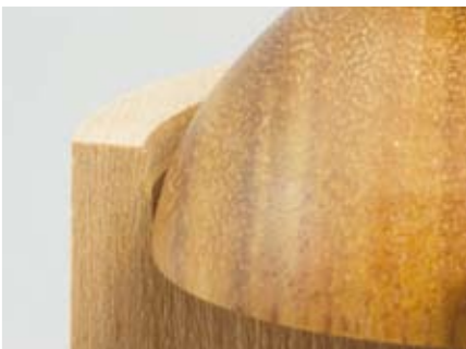
If you make a mistake and over cut, leave the mistake there. It will help you when making your next attempt. If you do need to remove it for access, do so after you have achieved the proper fit
