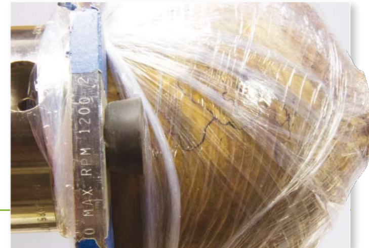
Stretch wrap works nicely to assist the Cole jaws with fastening the work to the surface. No adhesive fastening, just stretching around the jaws and over the work allows for more secure attachment. Mind the direction of rotation when wrapping
