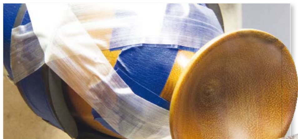
Tape on the bottom of the chuck and around the jaw faces allows for a gentle clamping. The painter's tape on the finished surface allows for the fibreglass reinforced tape to provide the actual strength for this mounting without damage
