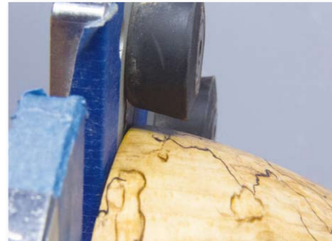
Turnings no longer perfectly round don't engage with all of the buttons on the Cole jaws. With the rubber bumper's durometer and the angle of engagement, even many perfectly round items can use some additional assistance in fastening
