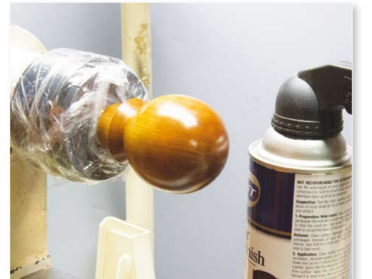
Stretch wrap works very nicely to mask areas off the turning or protect your chucks and other valuable equipment from paints and finishes. The low cost and ease of use makes stretch wrap a must have item in the workshop
