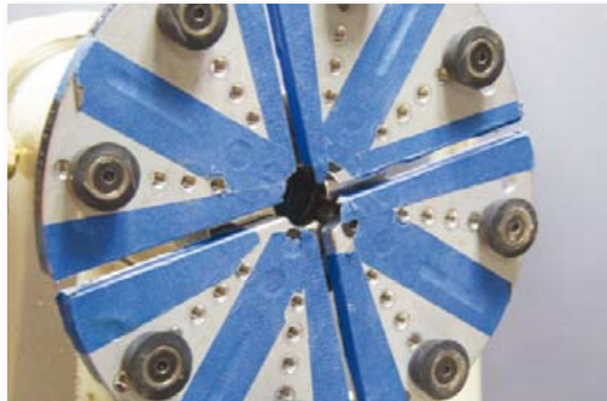
Since my Cole jaws always see a finished surface, I have a protective layer of painter's tape on the metal surface. Notice it is a uniform thickness of one layer in the area where the wood contacts the jaws
