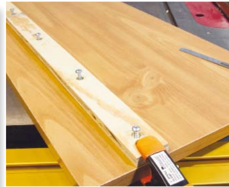
A single piece of shelving can be used for the table. I've favoured a front side of the lathe only position table but the lathe bed gap locator can be centred for work on both sides of the lathe
