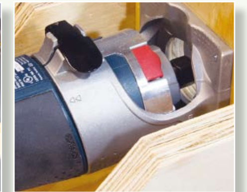
By designing and fabricating my Dremel adaptor plate to fit the hole pattern of the Bosch router base, I can position my Dremel to the same centreline as my router and any turning
