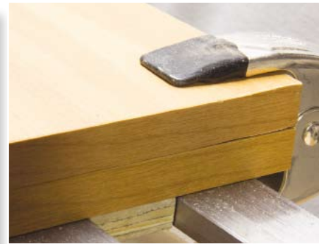
Since there is little loading on the table, you might find a squeeze clamp sufficient to fasten the table to the lathe bed ways. A good fit for the locator strip, or shorter blocks if you choose, secures the table nicely
