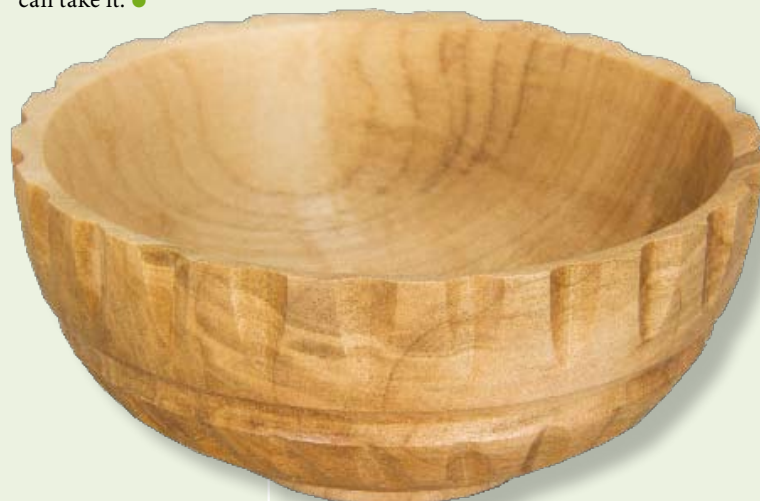
A simple bowl displaying a rotary cut, straight axial cuts, and slightly angled axially cuts with a cove router bit. What can't you bring to bear and where will you take the idea?
