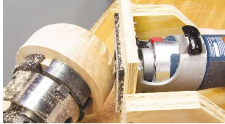
The depth stop is especially important when working on curved turnings. The router base, which would normally contact and control depth of cut on flat surfaces, doesn't work on curved surfaces
