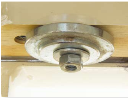
With the lathe bed gap locator intentionally thinner than the ways, almost anything can be used to clamp the table in place from fender washers to blocks of wood to clamps for other lathe accessories
