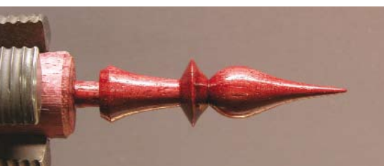
Assembled turnings give you plenty of freedom to create until you are happy. Notice the great grain orientation for gluing. Also, there is no grain match to speak of so any finial produced, #1 or #20, will blend right in to the final product
