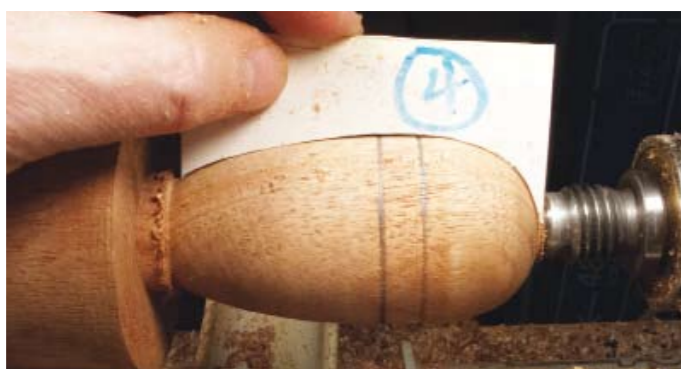
Having both complete and section templates makes easy work of this approach. Taking each section to completion as you progress towards the headstock. It is easy to be too critical when looking and working this close
