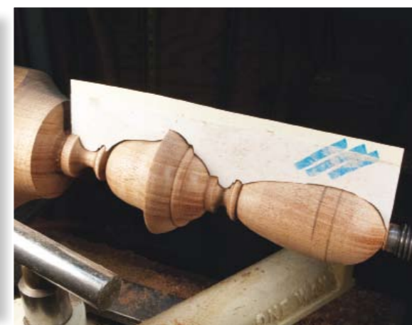
A final check prior to a quick sanding of the curves and removal of the end markings. While only making one in this instance, can you see where multiples become more doable with this technique?
