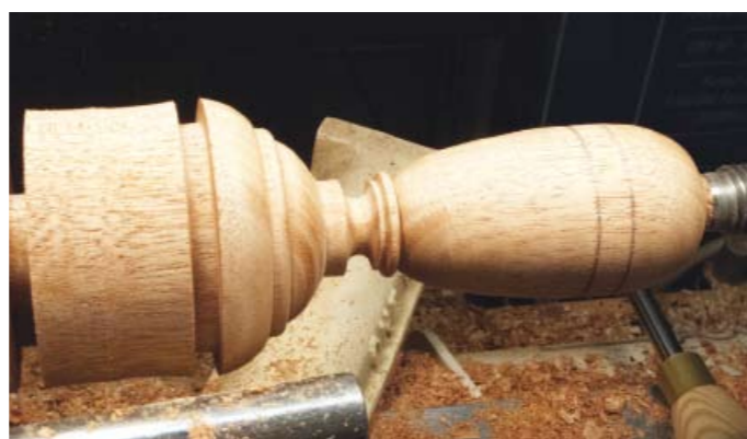
I like the modular approach to cutting to completion section by section. It helps me with the blending of areas and keeping things in the proper perspective
