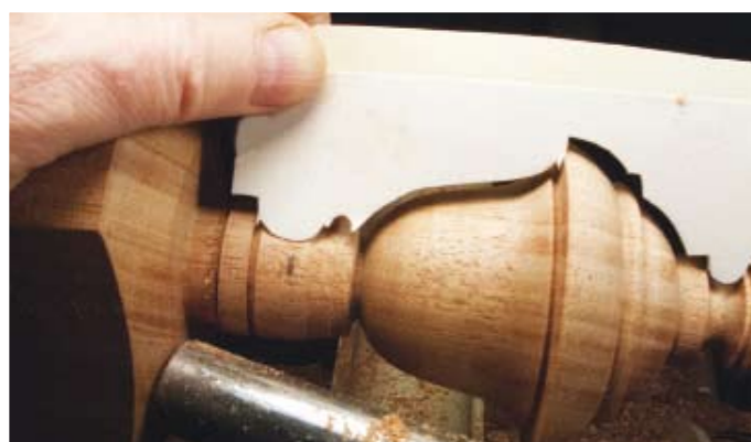
A spot check of the overall periodically will allow for any small flow problems to be corrected. If things go too far before being brought back into line, there is a tendency to lose smoothness and be abrupt
