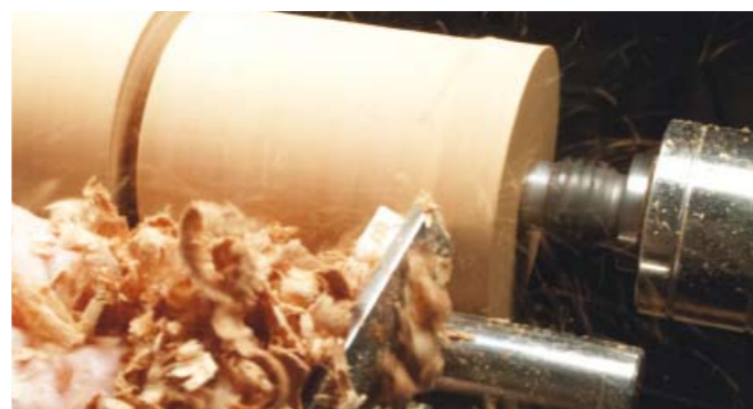
Working between centres, even though the headstock end is in a chuck, provides plenty of support and stability. Section by section work areas allow for focus and no defects forward mentality
