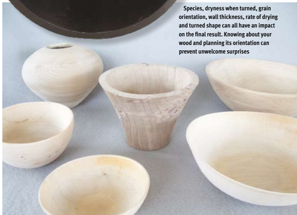
Every species has its own moisture coefficients in all three axis. The longitudinal, radial and tangential all interact with each other. The grain orientation in the piece will determine what the effect is
