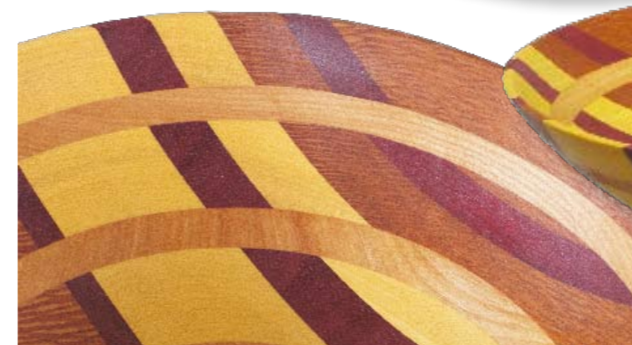
Of course, sometimes the rules can be broken or at least bent a bit. This multi-species glue up with all different grain orientations only survives – 12 years so far – because of the thin wall thickness. Thicker would likely fail
