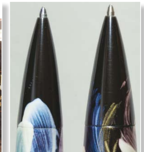
No finish can prevent the changes in wood based on moisture. The Corian nib to wood fit in both of these pens show the shrinkage of the wood during the winter changing to a less than perfect fit
