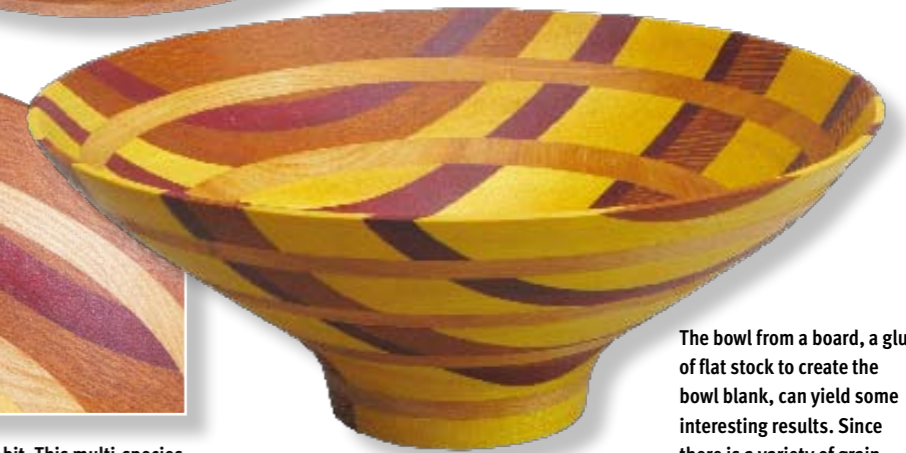
A different bottom treatment, avoiding end grain to end grain joints, in the bottom of this segmented bowl has worked much better. Attention to grain orientation is as important when gluing as when turning
