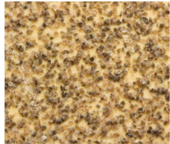
Sandpaper needs to be treated like every other cutting tool. Keep it sharp; that means throw it away when it has been spent. Go slow enough to keep the cutting edges in contact and cutting
