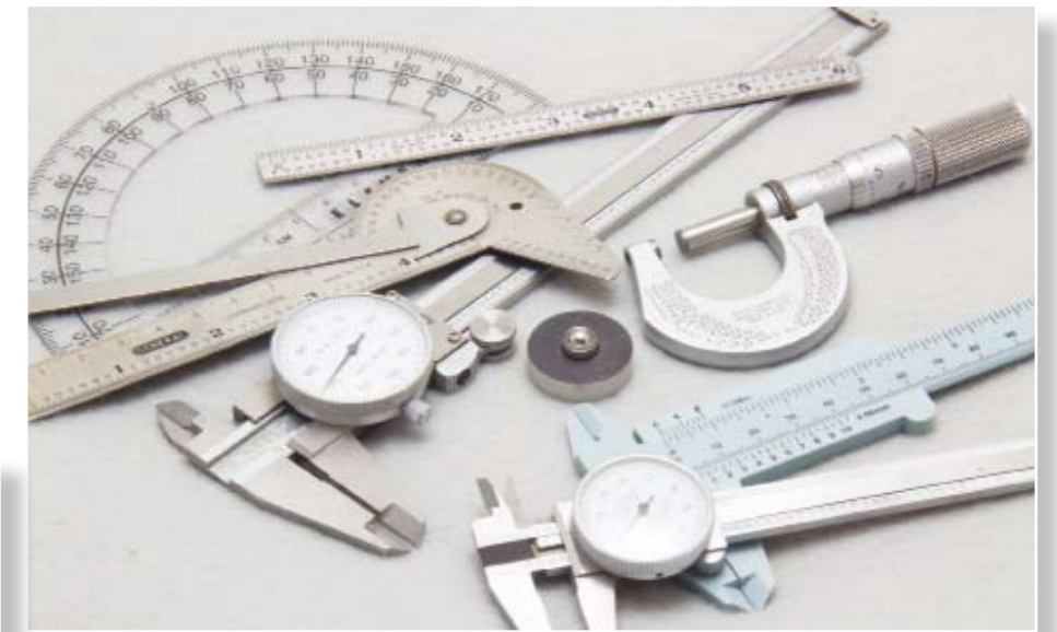
There are many types of measuring tools that can be used by the woodturner. While gauges yielding measurements are sometimes needed, more often the appropriate gauges are transfer gauges
