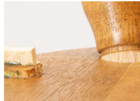
An example of fits where the diameter needs to be close so it can be seated with sufficient glue space but the tolerance isn't that critical. Fit allowing for glue but the spreader will lock it into place
