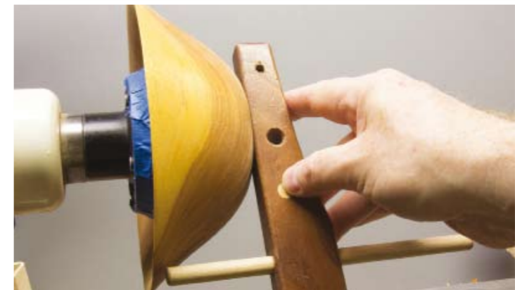
This homemade bowl gauge is useful both on the inside and the outside in helping keep them where they belong. It can show progress in hollowing as well as material remaining
