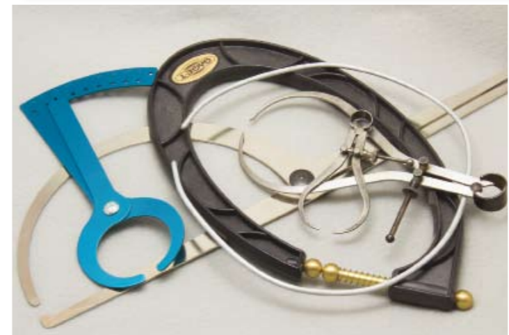
Just a few of the various gauges available to do wall thickness on bowls and hollow forms. They range from a bend wire or rod to purpose made thickness gauges with relative or units based scales
