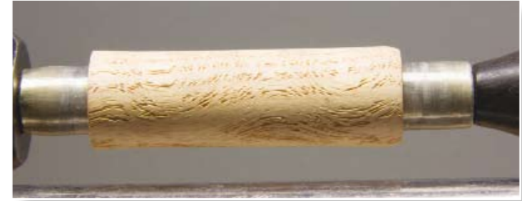
Pen turners often use bushings as their workholding mechanism and their gauging method. The wood is turned until it matches the bushing indicating that the proper diameter has been achieved
