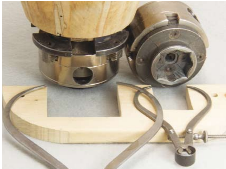
You can set your callipers as needed or perhaps set aside two callipers that are always set to the min and max for a chuck tenon. Much easier and less expensive is a cardboard or wood template
