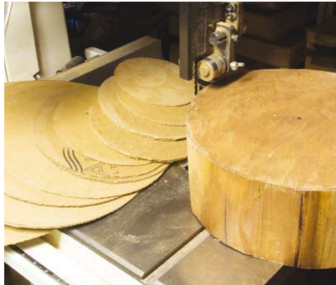
Whether flats or split logs, a cardboard template of the desired diameter will allow for the flat side on the bandsaw bed and a safe way to cut the bowl blank. Low cost, easy to use and replaceable
