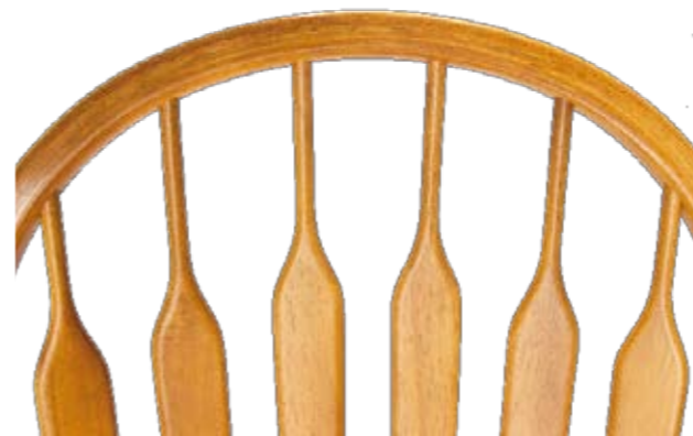
'Identical' items that are close together are difficult for most hobby turners. Even with templates, care must be taken since the eye isn't fooled easily. Can you spot the flaw in this chair back?
