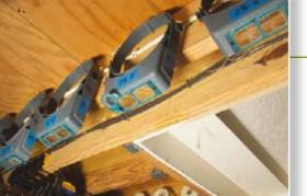
My Optivisors are all marked with the focal length, allowing me to quickly grab the set I need. I also include the sequence order and magnification on each label, but this is more for other users
