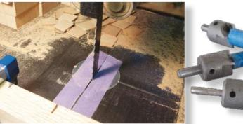
Low-tack painter's tape works well for everything from masking turnings for sprayed finishes to closing the size of your bandsaw's throat plate. Keep rolls of the tape at different locations throughout the workshop so that it is always to hand to solve any immediate problems
