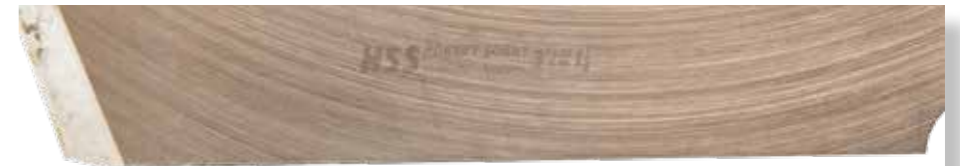
The most common tool steel used in the modern woodturning tool arena is high-speed steel. It is almost always laser marked somewhere on the tool as HSS
