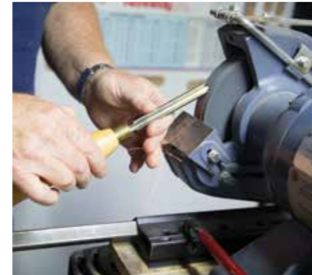
The use of jigs and fixtures can not only make the process easy and repeatable but can also let the newcomer focus on the many other learning needs
