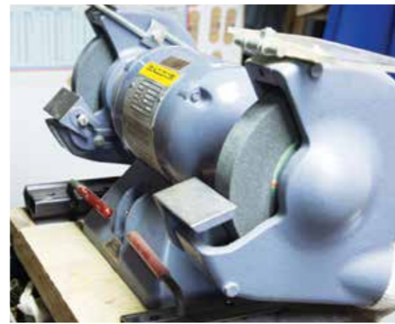
The sharpening system most commonly used is the bench grinder. A slow-speed grinder is more forgiving but modern tool steel isn't damaged with heat from a grinder
