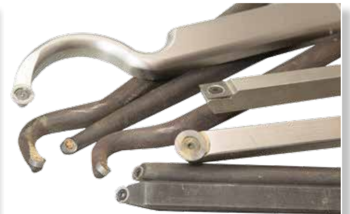
The replaceable cutter tools have been making inroads lately. The carbide cutter is rotated as needed to provide a sharp edge and replaced when totally spent
