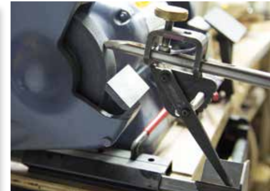
A well-equipped sharpening system will have quality toolrests and also provisions to accommodate jigs and fixtures for either regular use or those special needs
