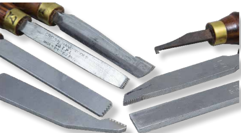
Hand-chase threading tools for different pitch threads, including inside and outside cutting tools along with the tool used to cut the inside thread run-out area. All of my threading tools were made by Crown Hand Tools
