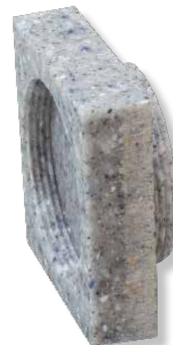
My start of an insertable set of matching threads. Using hand chasers, the inside thread is cut in Corian and then an outside thread from another piece of the same material is threaded being tuned to fit
