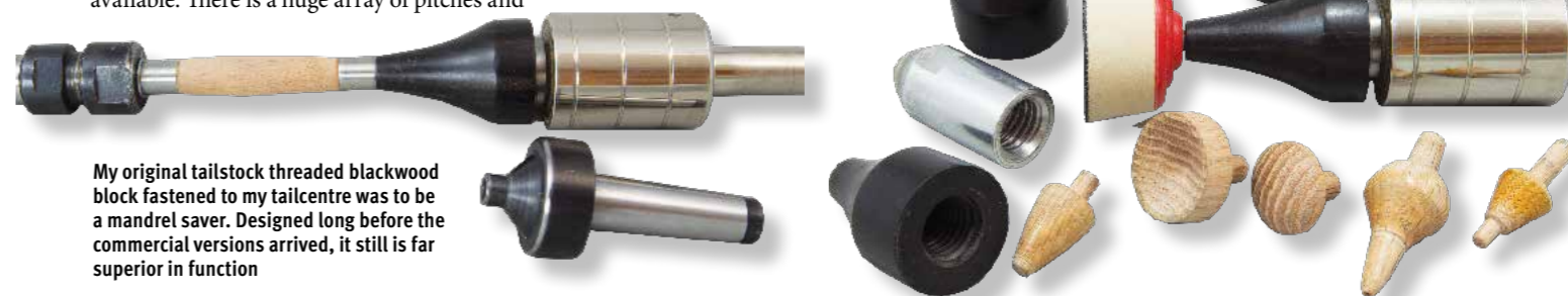
BOTTOM: Feel free to make a batch of headstock and tailstock accessories. My mandrel savers, metal and wood, accept sanding disc pads as well as a host of other special holders, pilots and friction blocks
