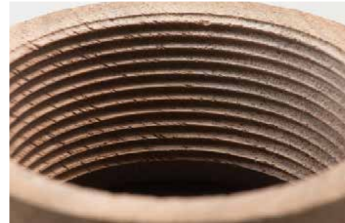
Threads can also be cut into the face grain like a bowl, as opposed to the usual spindle threading orientation. Weakness is still an issue and now comes the problem of expansion and contraction orientation
