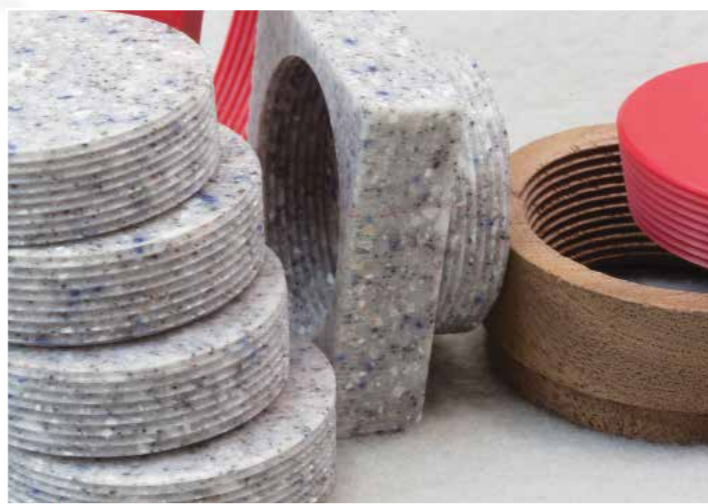
Hand-chased threads for inside, outside, or matched pairs are mastered with a bit of practice. You can easily do tapered threads as well. Like all woodturning skills, time at the lathe is needed
