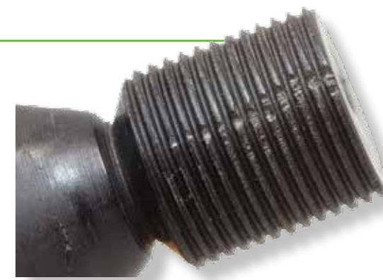
Even with dense, straight-grained woods such as this African blackwood ( Dalbergia melanoxylon ), the threads are still fragile based on the grain orientation with respect to the peaks of the thread
