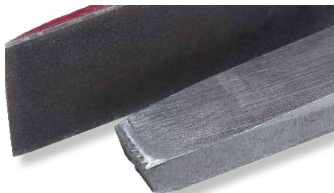
There are those who sharpen their threading tools on a grinder to freshen the top edge. I favour using a diamond hone. Laid at a very slight angle off top flat, a few strokes will provide a new edge
