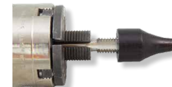
TOP: Standard machine-tool taps and dies will work nicely on wood. More readily found at the industrial supply house, nearly any thread is available. Common woodturning sizes are now coming into stores
