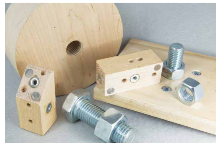
Whether threading the bowl blank for use or embedding nuts and bolts into jigs and fixtures, always be aware of the strength needed for your application. Always over design for the sake of safety
