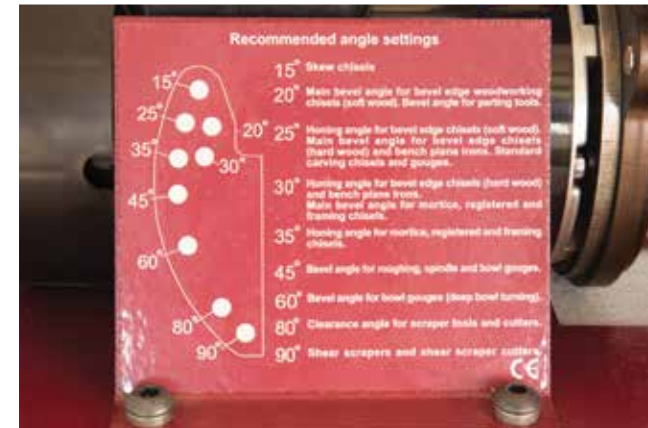
With every typical grind angle available by locating the pin in the correct hole, the chart on the front shows the pattern. It also explains the typical uses for each of the angles
