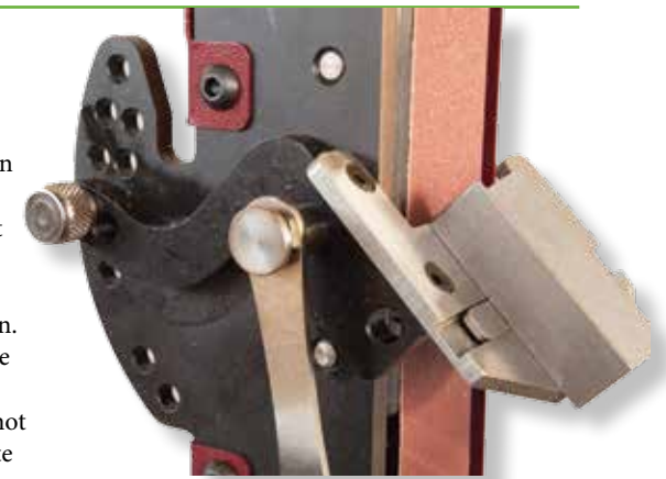
By design, the Sorby ProEdge has all of the commonly used grind angles built into the mechanics. This makes obtaining the desired angle a breeze but more importantly makes it very repeatable
