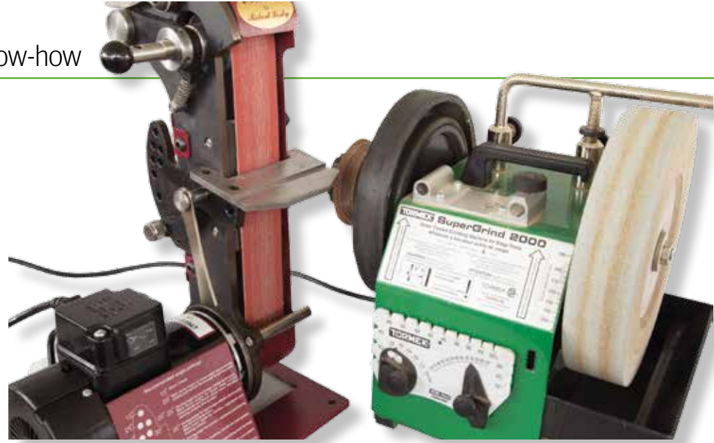
Moving beyond the bench grinder takes you into the belt grinder and water-cooled systems. The Sorby ProEdge and Tormek are the most prevalent of these types in the marketplace
