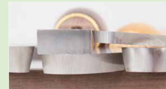
The advantage of the Sorby ProEdge and Tormek is their ability to deliver finely ground edges. Take a look at 60, 200, 1,200 and a mix of 60 and 1,000. The time and investment cost difference is your call
