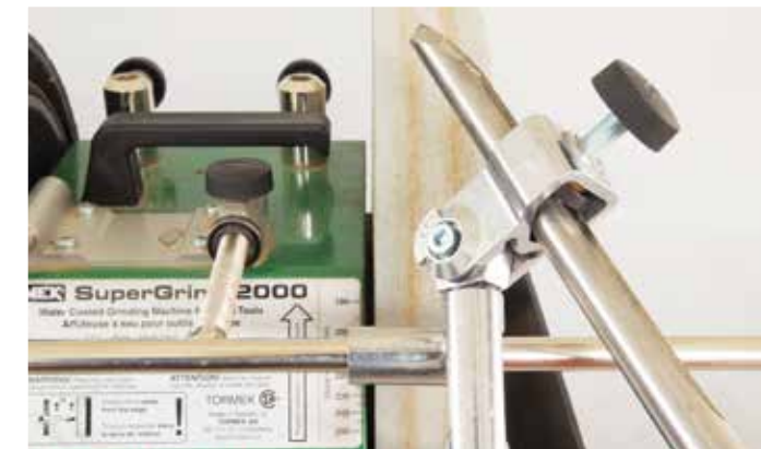
The Irish grind is possible using the Tormek jig. Once the user finds their favourite, the extension in the jig and guide-bar measurements are recorded and used over and over. It takes some easy measurement
