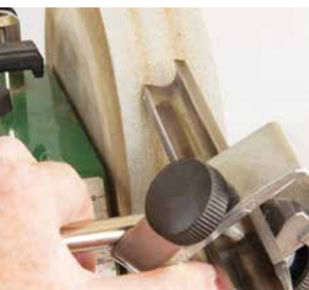
Not locked into hard position but being user adjustable, 45° or in that range is easily set on the Tormek. The setup jig makes the tool extension and the guide bar positioning quick and easy
