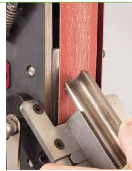
As discussed in prior issues, barring special needs, use 45° for most cutting tools. The 'V' block fixture riding in the platform with the Sorby machine set for 45° is quick, easy and repeatable
