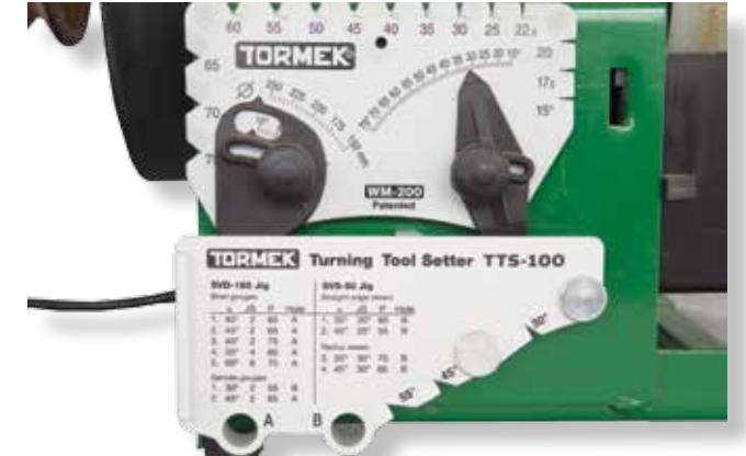
The Tormek adjustments are measured and locked into place. The new style gauge, lower, is far easier to use. Either will let you adjust the guide bars and jigs to your desired relationships. Infinitely flexible
