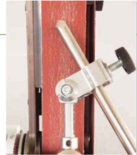
Setting the bowl gouge into the factory-set jig yields the swept back bowl gouge grind. An optional pivot block will provide additional length sweeps on the wings. Quickly setup and very repeatable
