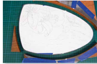
Using a photocopy of the master pattern, the tray blank is cut from the padauk material on the bandsaw. Minor stock is left proud of the pattern to refine the actual edge at the belt sander
