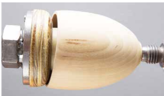
As covered in the working series, a friction drive can be made to suit nearly anything. Here, one of my vacuum chucks works nicely
