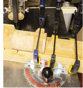
With the tenon cut for the upcoming chuck mounting, a stop block is clamped in place as is the cup blank after the fence is set for the desired angle. The flats intentionally left make a 'V' block unnecessary
