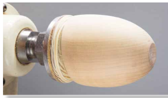
The only disadvantage of cutting the angle across the lip of the cup early is the inability to use a jam chuck for reverse mounting. There are other methods though, including a vacuum chuck
