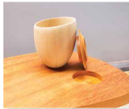
The beauty of additive processes is the error recovery potential. The cup nest, trial-and-error fitted, can be made as many times as needed with minimal loss of time and material
