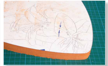
Using photocopies of the 'master' drawing, the pattern is fastened to the tray material and the shape is cut on the bandsaw. It's important to mark the centre point of the cup nest prior to removing the pattern
