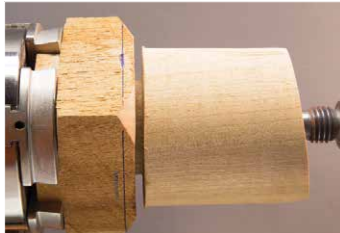
Mounted in the chuck with daylight at the bottom, the tailcentre is used as good practice. The absolute bottom is marked as is a cut to the diameter at the bottom of the cup at the nest interface
