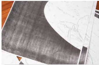
Because of the limitations of my copier, I need to make copies in halves and tape them together. Checking for dimensional integrity, the tape-ups are fastened to the stock for cutting
