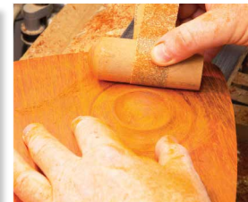
With only a small lip to be removed, sandpaper wrapped around a similar radius mandrel is used. The surface will be further prepped for lacquering
