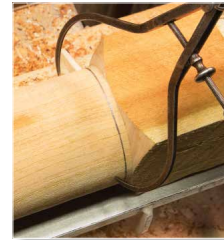
The blank is turned to near the maximum diameter and marked for the angle cut start position and absolute bottom of cup. Flats are left intentionally to allow for safe cutting on the bandsaw
