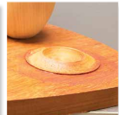
The cup nest, trial fitted in the Forstner hole and cup bottom, is wetted with some wood glue and dropped into place. A weight on top holds it flush until cured
