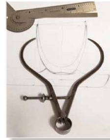
The angle of the cup lip is measured for planned processing as is the maximum cup diameter for selection of stock. Simple and effective measuring tools with no numbers really needed, just settings
