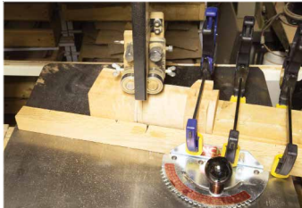
From a precision and safety aspect, it doesn't get any better. No hands needed to secure the stock as the cut is made and cutoff material is free to separate without restriction
