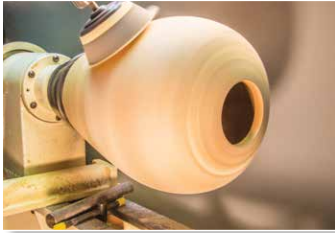
The sanding zone for the outside of a turning when the rotation is reversed and the turning is spinning clockwise
