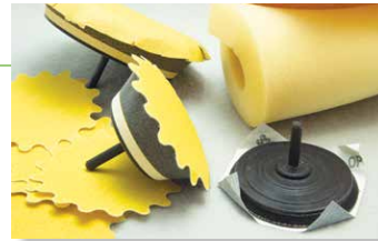
There are savings to be had cutting your own pads and sanding discs. Whether scalloped or folded up edges, you can soften the sanding process and cornering
