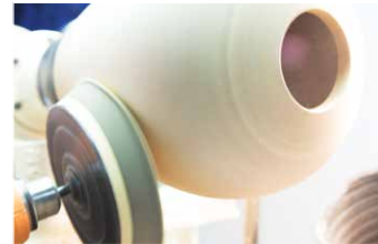
Power sanding position on the outside of a turning with the lathe running counter-clockwise or the normal turning rotation. Be careful with large pads and small shafts
