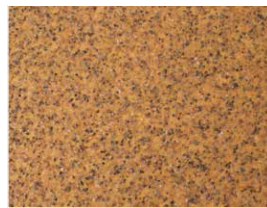
Think of sandpaper as a cutting tool, much like your lathe tools. Each particle of abrasive works the same as your tools
