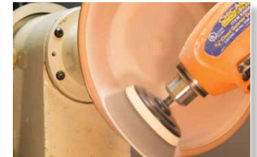
A good sanding zone for sanding, powered or not, on the inside of a turning when the lathe is running counter-clockwise
