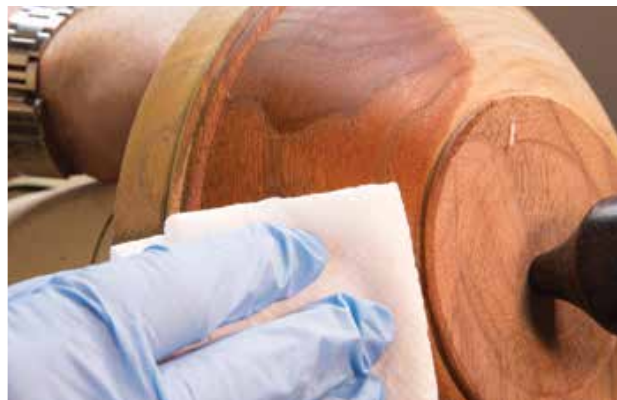
With proper PPE, a quick wipe with mineral spirits will often show sanding flaws easily overlooked on the turning. Mineral spirits won't raise the grain
