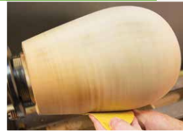
The safe zone for hand-held abrasives with the lathe running normally is at the seven to eight o'clock position. The abrasive can be safely pulled away and the hands won't jam
