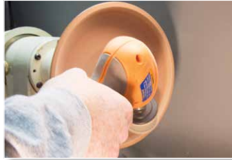
The sanding zone for the inside of a turning when the rotation is reversed and the turning is spinning clockwise
