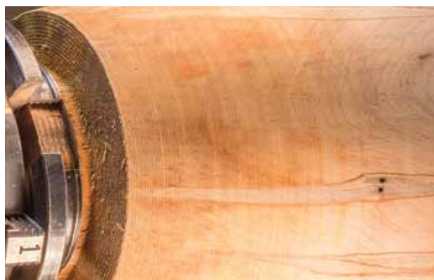
The coarsest grit of abrasive is used to remove the tool marks. Start where you need to with your abrasives. Starting too fine won't be effective
