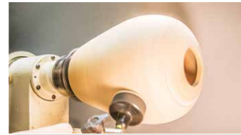
The non-powered rotary sanding pad gets its power from the rotation of the part. After learning the knack for getting it running, you'll enjoy using it
