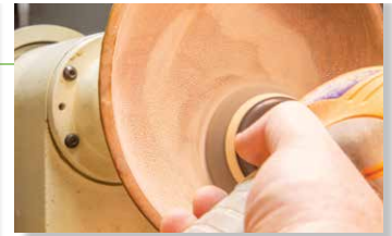
Stopping the lathe lets you attend to areas needing special attention and use the pad flat. This is combined with normal power sanding as needed
