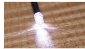
Examine the surfaces as you go with a high angle of incident light. If you missed any scratches then go back to the grit that you need to be able to correct the problem
