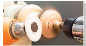
The various stropping and rotary sanding brushes work nicely on carved and textured areas. They will sand without significant loss of detail or digging
