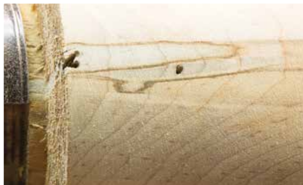
Once the tool marks are gone with the coarsest abrasive grit, each successive finer grit removes the scratches from the prior grit. Keep going until your level of scratch 'invisibility' is reached
