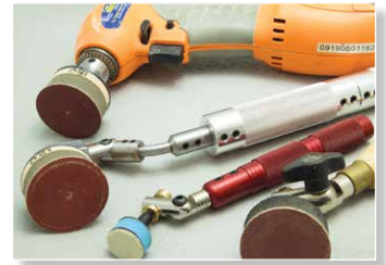
In addition to the powered power sander, there are many sizes and versions of the non-powered, rotary sander using the turning rotation for power
