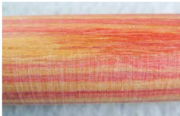
Don't be afraid to stop the lathe and sand with the grain. Using the same grit will make a marked difference. Do this at each grit if necessary
