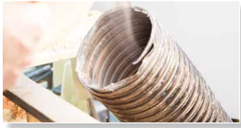
Dust extraction at the point of creation reduces the amount of sanding debris that is cast into the air. Personal protective equipment such as a dust mask is still recommended
