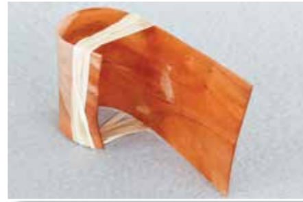
Rubber bands can be used to hold shape once bent but also can be used as a bending aid by tensioning then wetting and heating
