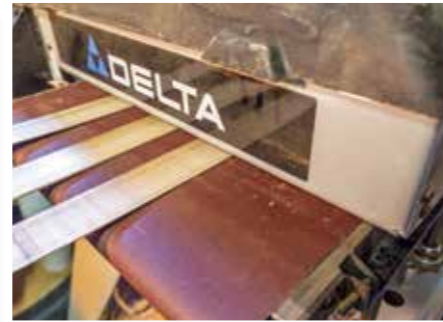
Depending on your end goal, it is easiest to sand your stock prior to bending. It bends better and is far easier to sand in the flat state
