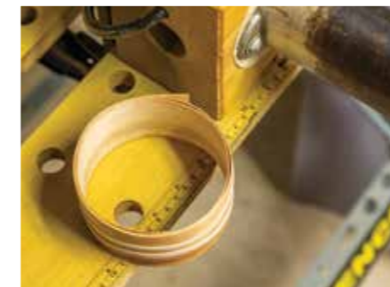
The thinner the stock, the quicker it can be bent and the tighter the radius. This 815mm length of maple is bent into a coil of 100mm in diameter
