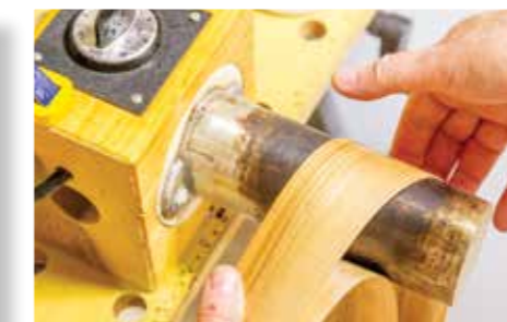
Work the wood! This is a progressive process of wetting, heating, wetting, heating, coaxing the form and repeat until it gently yields to your wishes
