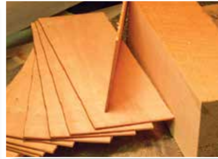
While nearly any species can be bent, some bend easier than others. This 100 x 100mm block of cherry is resawn for bending. Cherry and maple bend nicely
