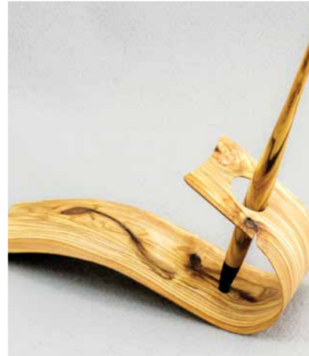
Steam-bending works best with regular shaped wood. Add contours, holes, scallops and other features after the bending is completed
