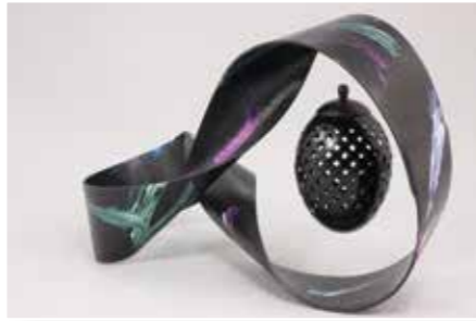
This ornament hanger is created by steam-bending a length of wood into a coil shape so it can be completely steamed at once and then twisted into shape
