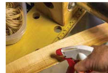
A misting spray bottle with plain tap water is all that is needed to wet the wood. I have found that soaking ahead of time didn't improve success at all
