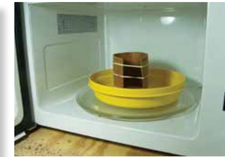
A household type microwave will work. Do not use for food service ever again once you've used it for drying or bending wood
