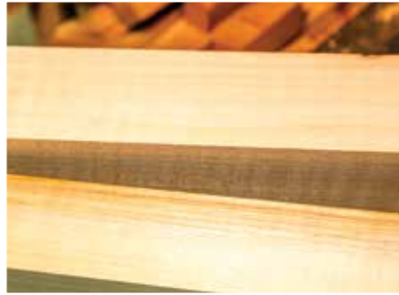
Material selection will make or break your steam-bending efforts. Here soft maple is selected for resawing because of the straight grain with no figure
