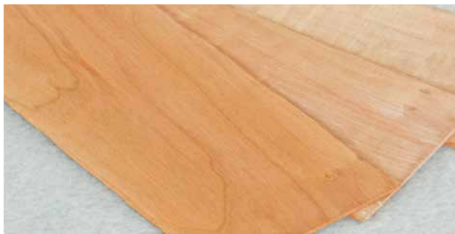
Good, better, best from right to left. Removing saw marks will reduce the sites where fractures will start. Rough sawn can be bent but requires more care
