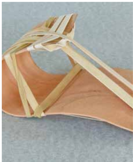
The meagre rubber band is an incredibly versatile clamp. By twisting, stretching and controlling contact points, you can perform clamping like no other
