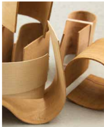
Regardless of the material and the ultimate shape, if the grain isn't perfectly oriented to the surface of the wood it is likely to fail, now or later
