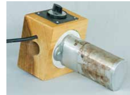
Made for instrument makers, this luthier's iron is made for bending the sides of a guitar. Different versions are made for everything from violins to basses
