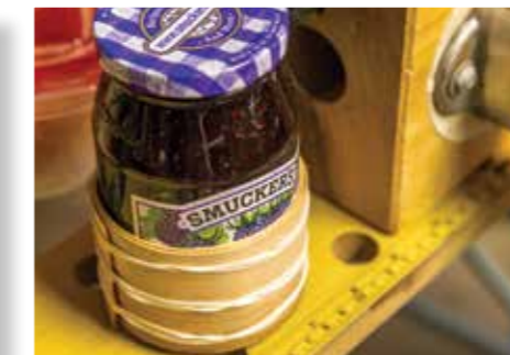
If you want to ensure that the coil is perfectly round, use a form of some sort. This jam jar works nicely and creates a perfect circle of 75mm in diameter
