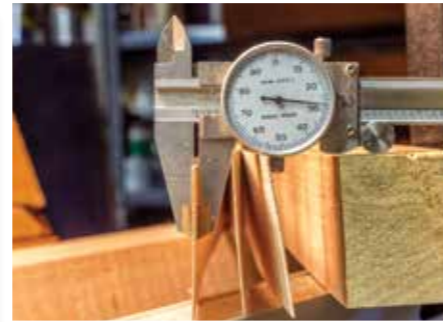
With a well adjusted thickness sander, you can easily get to a finished thickness of 0.8mm or less. The thinner the stock, the more successful you'll bend
