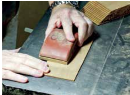
If you don't have a thickness sander or the stock doesn't lend itself, there is nothing wrong with hand sanding or using a card scraper
