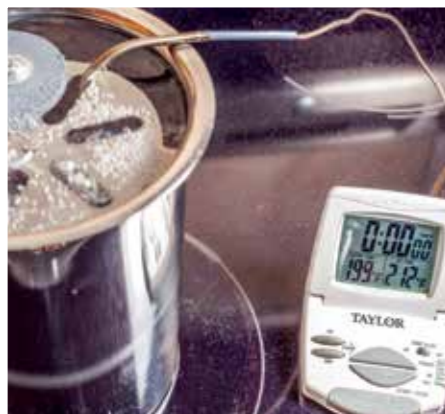
My off boil is at 199°F, which is perfect for curing the stabilising resin. A full boil at 212°F. makes for a mindless temperature process
