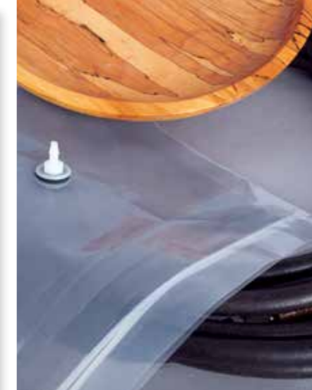
Help yourself with vacuum bagging by creating a cradle to minimise bag filling dimensions. My air line coiled up works nicely
