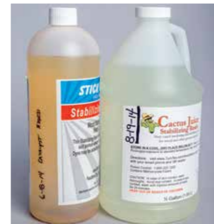
Don't catalyse until needed and then mark clearly. Use old stock first for best results
