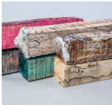
Unstabilised blank, lower front, with all others stabilised. Top front, as done, with the rest bandsaw faced to expose results
