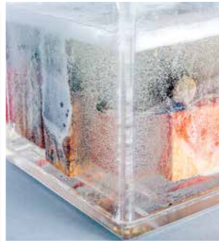
You can monitor the process until the bubbling diminishes to almost nothing. Keep sufficient resin for submersion
