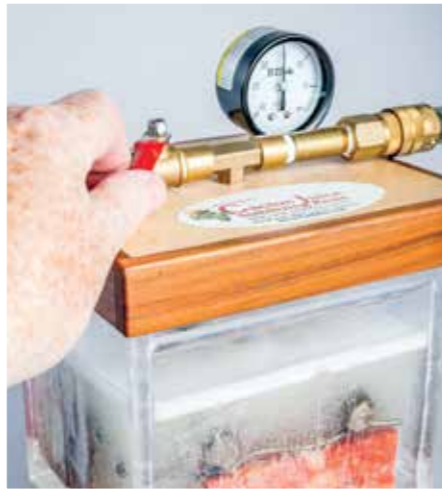
Slowly introducing the vacuum will minimise foaming and stresses on your vacuum system. Increase to full as needed slowly
