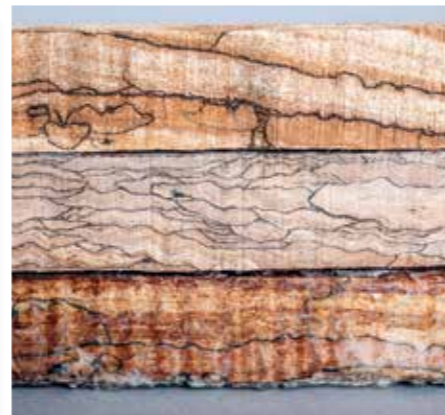
Taking a beautiful yet fragile blank, on top, and densify it for use is a joy. Underneath, both are ready for detail and long life
