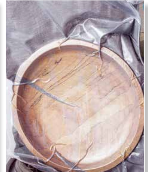
With sufficient resin for absorption, the bag is pulled to full vacuum with care to provide for a liquid trap
