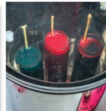
Use smaller containers for dyeing; this will help you to minimise the amount of resin to be coloured
