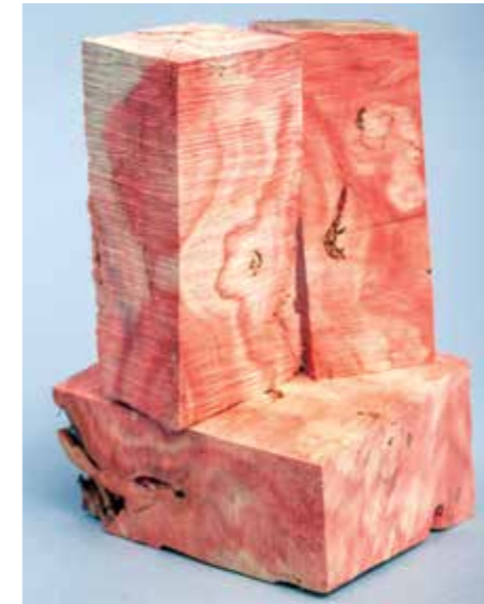
Boxelder ( Acer negundo ) burl cut to size for processing. The stabilisation will toughen it for turning and also help keep the colour from fading
