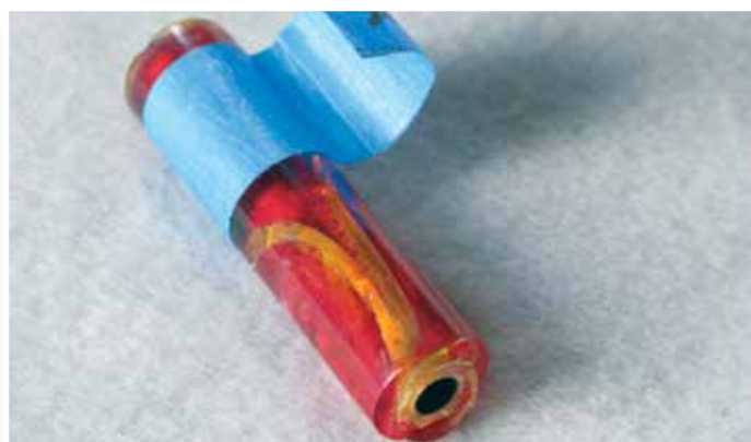
With care, embedded material plastics can be turned and finished. High speed, light touch and cool processing will be the keys to success
