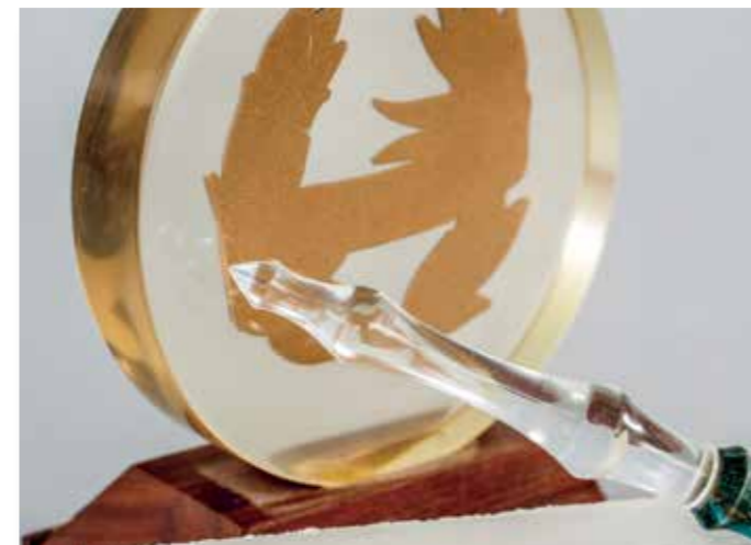
A good source for clear acrylic is old trophies. When cut, the material frosts. With proper sanding and buffing, it can be brought back to optically clear
