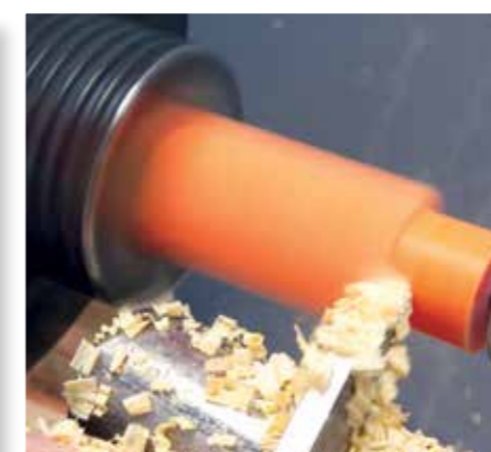
A sharp parting tool will work very nicely, not only on tight spaces, but also in the open. Basically a skew chisel, it will create very nice straight sections
