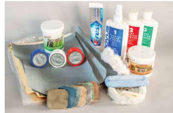
In addition to standard abrasives, a set of Micromesh, buffing wheels and media, and the various compounds with minute abrasive particles are helpful
