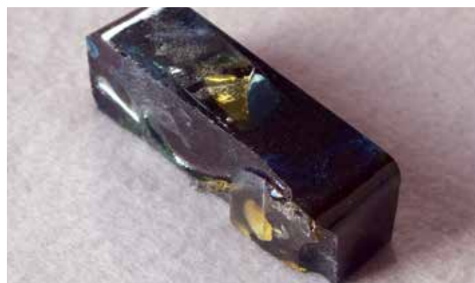
Embedded materials for colouring, as opposed to chemically altered, are a separation waiting to happen. Use caution when processing. Be gentle!
