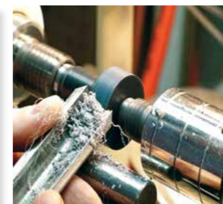
Thermosets are easily worked with cutting tools. The material cuts nicely with whispy curls possible, which creates a very nice surface finish
