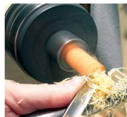
Depending on the hardness, plastics will hold nice detail – especially thermosets. A sharp detail gouge will work quite nicely to cut in features
