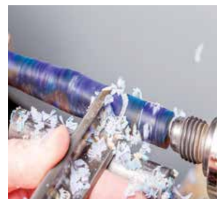
Thermoplastics usually like cutting better than scraping. A spindle roughing gouge works quite nicely if sharp and presented properly
