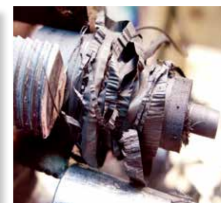
In contrast, a piece of Ebonite after a bit of heavy-handed turning. Plastic is worked far better with light touch and sharp tools. No need to beat the materials
