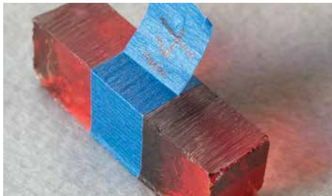
The chipping on the edges gives an indication that this might be brittle and chip easily when cutting. The number label helps me keep track of material batches
