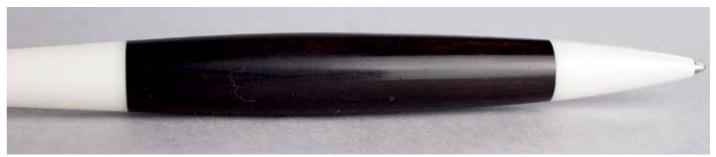
Bare wood can be buffed as can plastic. The lower portion of the Blackwood barrel is buffed only, no wax. The difference is apparent
