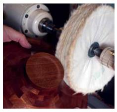
Keys to good buffing are: let the compound do the work, always work off the edges and keep the work moving
