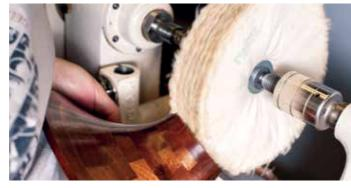
The key to good buffing is to use a mild pressure and let the compound do the work. When buffing, always keep the work moving to avoid burn through
