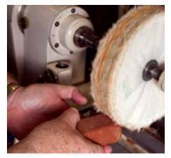
Charging and recharging the wheel with buffing compound is a simple task. Done below centre with an easy touch, the wheel is lightly loaded for use
