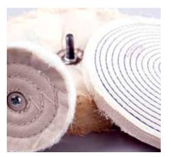
Buffs are available in different materials, diameters and rigidities. By stitching the buff, the pattern and nearness to edge controls the stiffness
