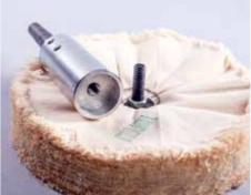
I favour the version that mounts in my lathe. The adaptor fits into the taper and provides the proper threading to receive the various buffs
