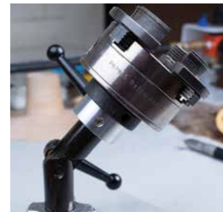
With the correct adaptors, carving vices and other adjustable workholding equipment can receive your standard lathe workholding devices
