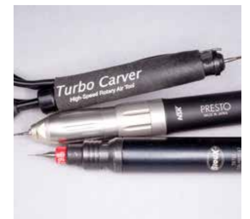
A machine tool grade die grinder and my two favourite high-speed tools. The die grinder is used with thicker materials and the high-speed tools with shell and thin stock
