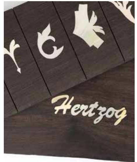
My practice pieces in mother of pearl cut and inlaid. Inlay can enhance flat surfaces regardless of the inlaid material and smaller can be done in the round
