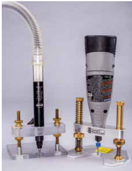
Where depth of pocket is critical such as inlay, a luthier's purfling attachment can be used. They are available with many different rotary tool mounts
