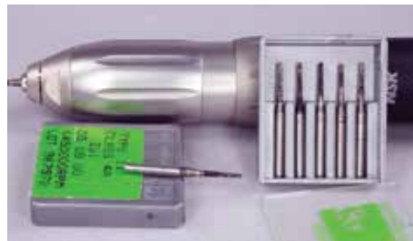
My most used tool and piercing bur design. Notice the manufacturer's speed limit maximum at 450,000rpm. Always heed the cutter and bur speed limitations
