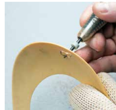
The slower micromotor tools with their beefier cutters work well in thicker materials. The slow speed minimises any burning
