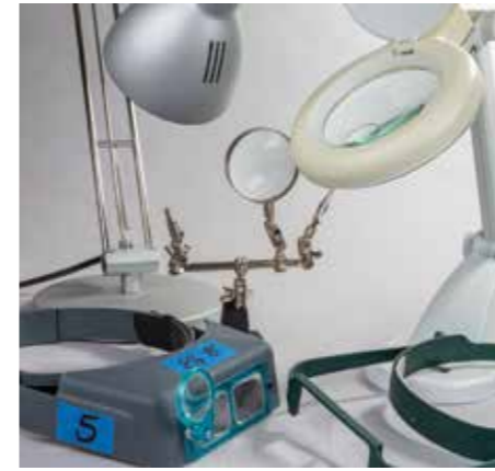
The naked eye can be aided considerably with good light and magnification. Whether head mounted or magnifiers sitting on the table, any of these help
