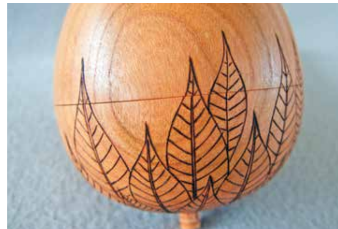
A cherry ( Prunus serotina ) lidded box body with desired leaves pattern burned into surface and now readied for colouring with alcohol dye markers
