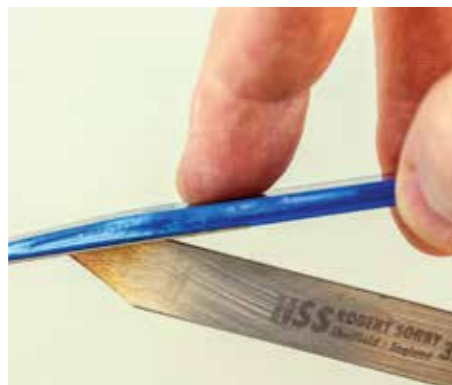
Using the back edge of the hollow grind as support, the front edge is found and contact with both is maintained during honing
