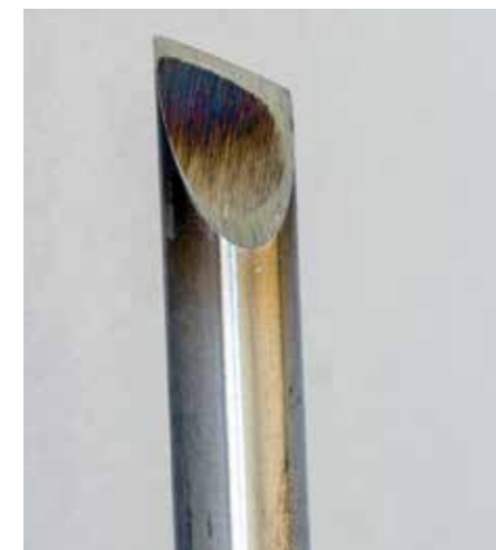
Round skews are simply a skew grind on round stock. Using a hollow grind allows for easy sharpening with a diamond hone
