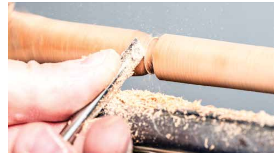
A round skew can be used exactly as any other skew chisel. The size and shape lends itself to smaller detailing and bead work
