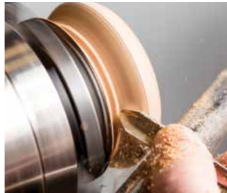
The shallower angle grind makes it easy to cut into tighter spaces without worrying about hitting the top edges
