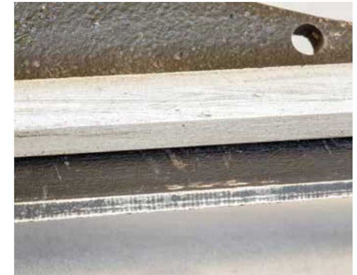
Even a new rest on the bottom can be improved by filing and waxing. The rest on the top will provide far smoother tool movement
