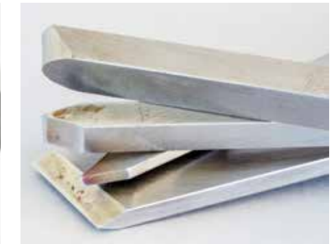
I soften the edges on all of my square cornered tools the moment I purchase or make them
