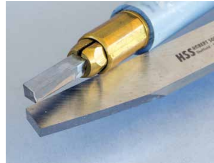
Modelled after the traditional box corner cutter, this high speed steel tool blank is ground to cut corners. Fastened in handle for safe use
