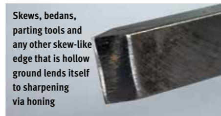
Until the hollow grind is nearly honed away, this honing method will work quickly and effectively
