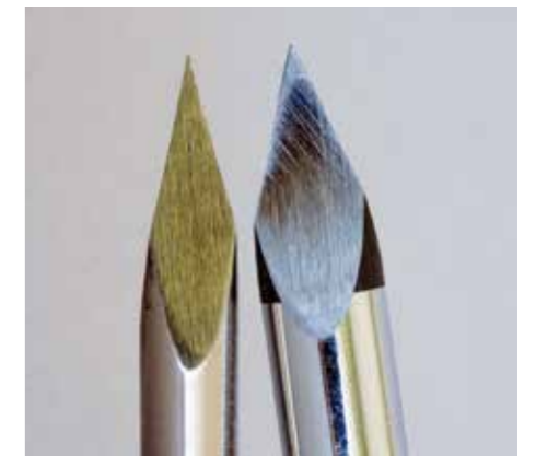
Commercially available, left, and easily made by the shop handy turner, tri-point tools are wonderful for detailing
