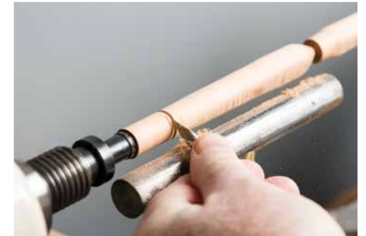
The tri-point tool is not only capable of V cuts and corner detailing but also rolling beads. Keeping the point clear is critical
