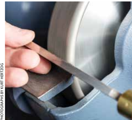
I use my grinder to soften the sharp corners. One sweep from ferrule to end of tool at about 45°
