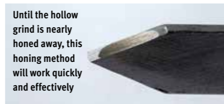
Skews, bedans, parting tools and any other skew-like edge that is hollow ground lends itself to sharpening via honing
