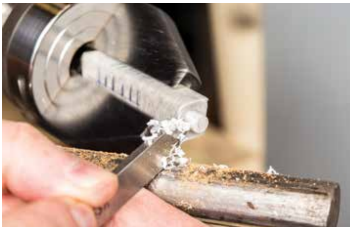
The off perpendicular angle allows for cutting a true 90° corner or angles less than that. I use it for concave corner interfaces
