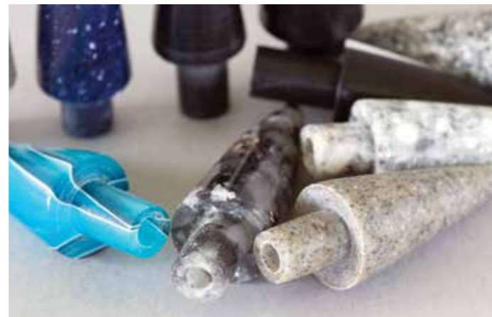
Whether my nibs are in Corian, other plastics, or wood, I use my off 90° ground parting tool to create the interface surface
