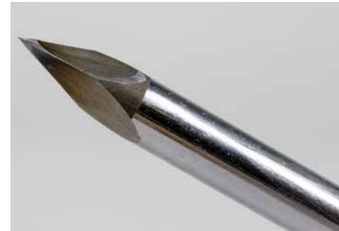
I favour mine hollow ground rather than the more common commercially available flat ground because I can use the honing method of sharpening more easily
