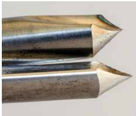
My standard spindle gouge, top, is ground to about 45°. My 'go to' detail spindle gouge is ground to fit into smaller spaces
