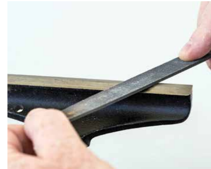
Removing dings and divots in your toolrest are key to smooth turning. Filed at 45° in one stroke, repeated until done, will clean up problems
