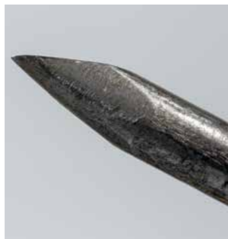
The balance of the ground edge is a convex grind. It needs to be controlled into cutting and will stop with relaxation of that control
