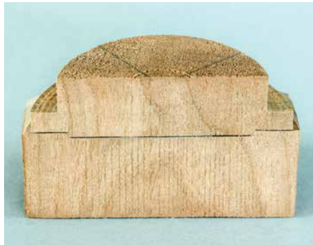
With compressive loads relying on the joint design, hot-melt is reversible with denatured alcohol
