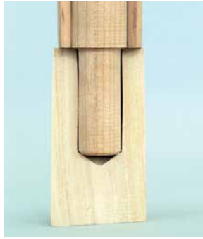
An added decorative ring can be turned separately and added as desired by sliding it over the diameter
