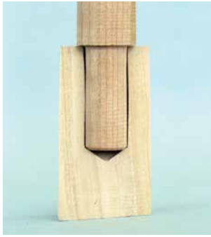
Depending on your choice, you can shoulder on the bottom, shoulder or both to provide column strength
