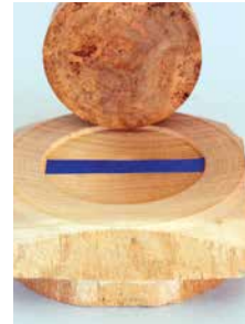
In order to minimise stress on any adhesive attachment, you can apply adhesive in the area denoted by the tape
