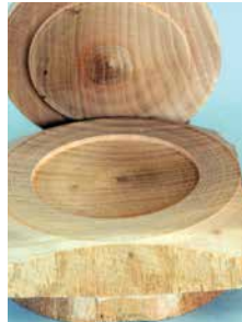
Any misorientation will put undue stress on the joint. Even different species should be orientated as best they can for grain
