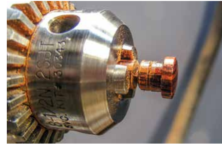
A glue trap groove cut into a pen end cap replacement. Adhesive is only to be applied to the lowest flat ring
