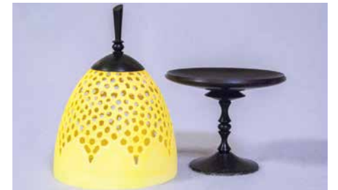
Base made from three pieces is commonsense based on ease of workholding and material cost savings. The finial is made from two
