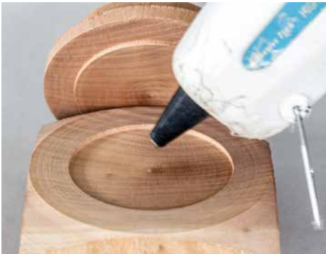
When the adhesive needs are only to keep things in position with strength from the joint, hot-melt can be a choice
