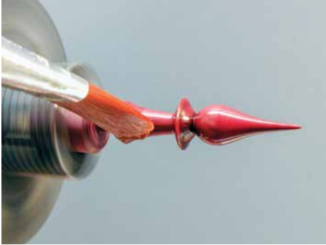
Finishing individual pieces as they are created has the advantage of not creating radii of finish in the seams
