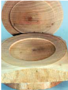
Keeping grain orientation for joint and adhesive bonding will help minimise stresses over the life of the turning
