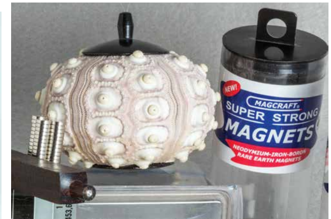
I've been using rare earth magnets glued inside my lower ornament body. A finishing nail head is embedded in the finial before turning
