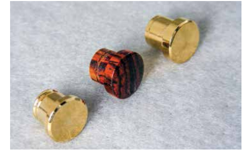
Because the wooden end cap can't be a hard press fit, it needs to be adhesively bonded but is susceptible to squeeze out
