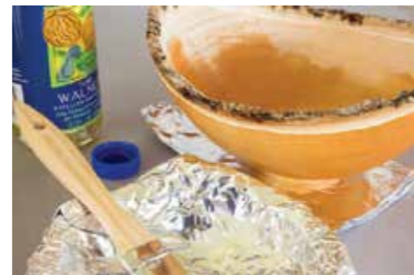
Applied liberally from the outside, it will wick into the wood and usually show up on the inside surface
