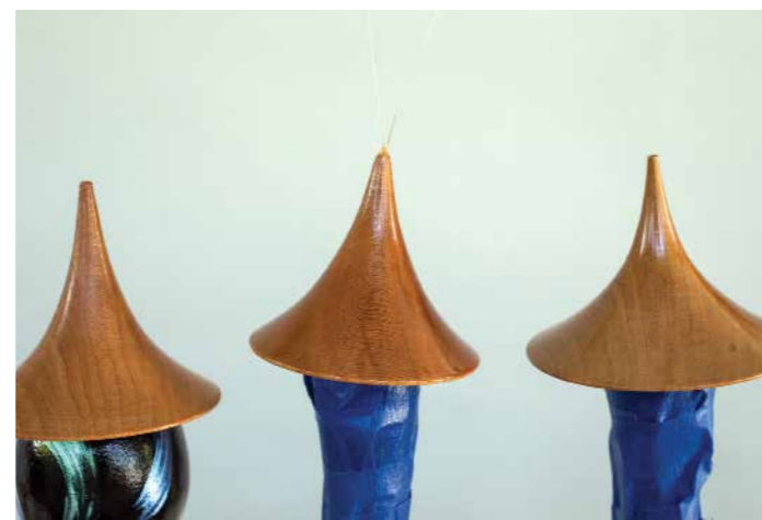
Some of my applications for shellac. Left – shellac matted back with steel wool; centre – shellac alone; right – shellac undercoat for lacquer top coat
