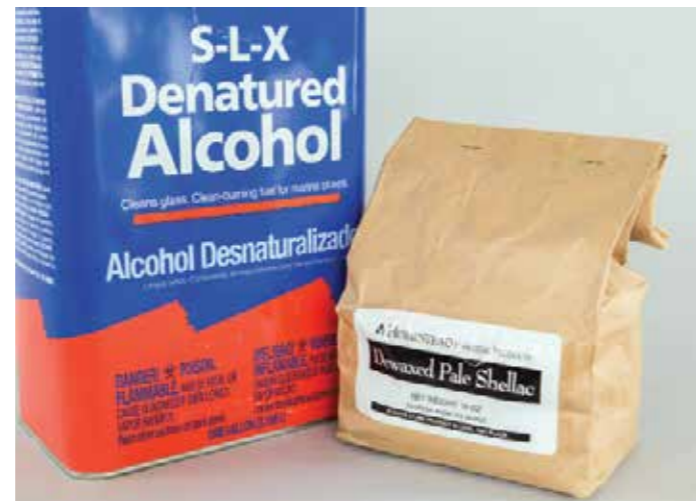
One pound to one gallon or proportional fractions thereof yields a 1# cut. Heavier cuts, i.e. 2# or 3#, use the added pounds of shellac to a gallon
