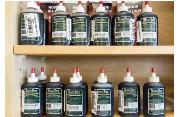
The colour options for mixing alcohol soluble dyes into shellac are endless. Mix and match colours and intensity to effect toning
