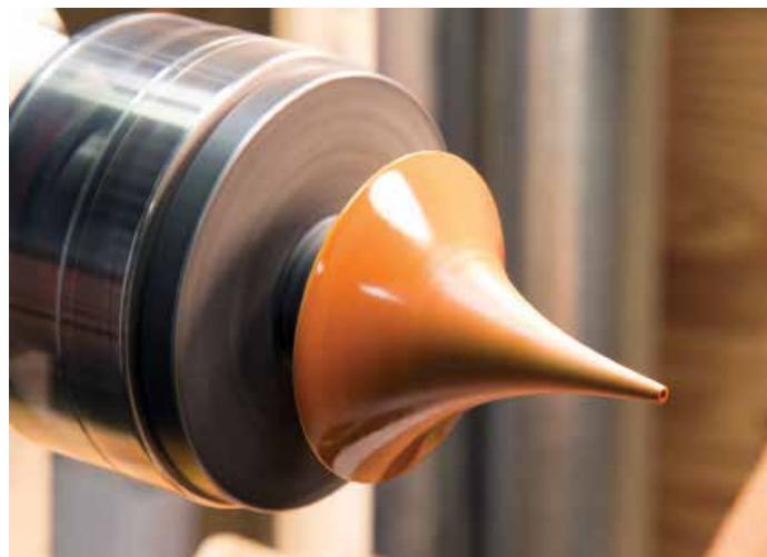
I usually spin the wet coats in the lathe to prevent any drips or sags that can occur with heavier applied coats
