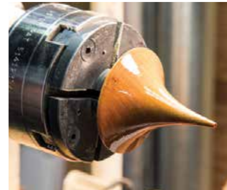
First coat of shellac applied generously by foam brush from a three pound cut of Zinsser Bulls Eye Clear
