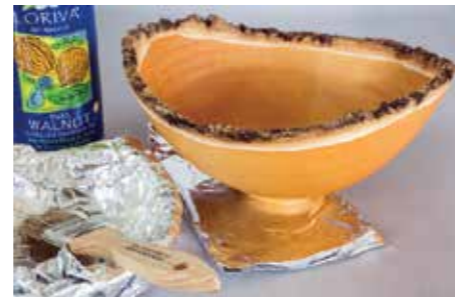
I don't usually count on an even coat on the inside from wicking alone. I apply coats to the inside in the same manner as outside
