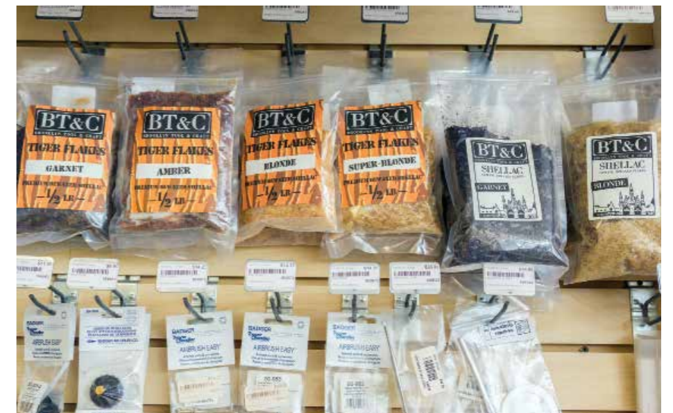
Shellac flakes are available in a variety of processed levels including waxed, dewaxed and different colour tints
