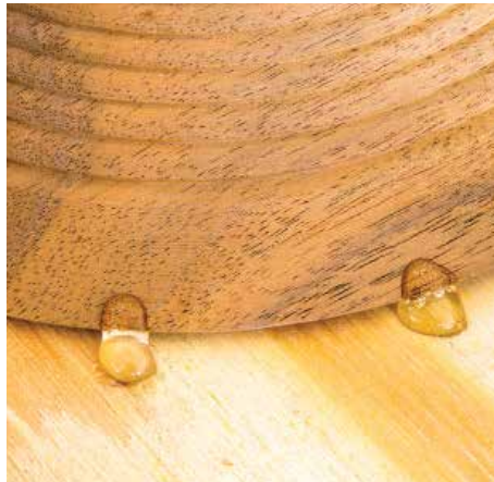
Some hot melt glue dots will fasten your turning to your wooden faceplate, just a few dots will do
