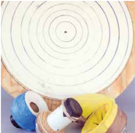
For the shop handy, vacuum chucks are easily made. Here from 1½ to 15 inches
