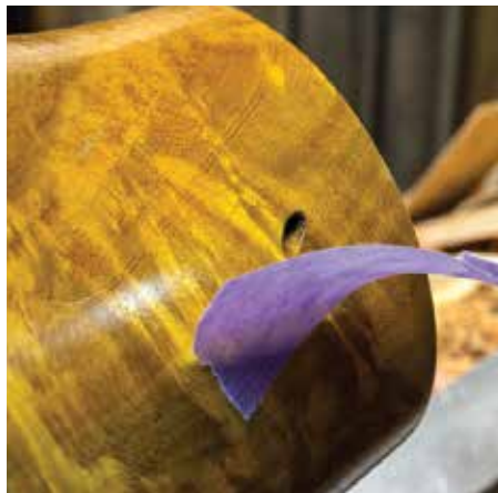
Most small vacuum leaks can be fixed with low tack tape or stretch wrap covering
