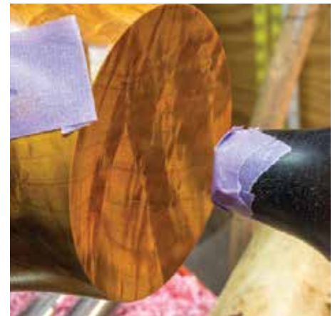
Regardless of your mounting method, use of the tailcenter is wise for as long as you can
