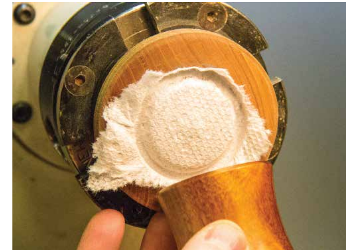
Making the jamb chuck fit loose and using tissue helps with easy removal, avoiding marks on the finish
