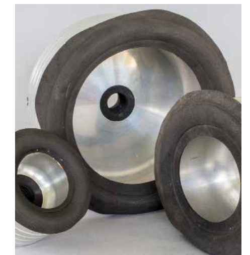
Changing from a 90mm to a 200mm vacuum chuck will magnify the force by a factor of five for the same vacuum
