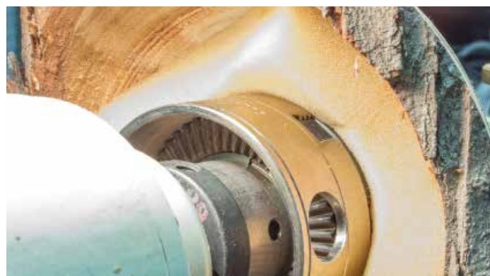
A foam pad over the jaws of the chuck is all that is needed along with the tailstock
