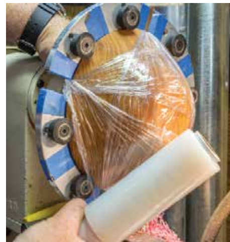
Stretch wrap packing tape works well for low stress mounts and for 'insurance'
