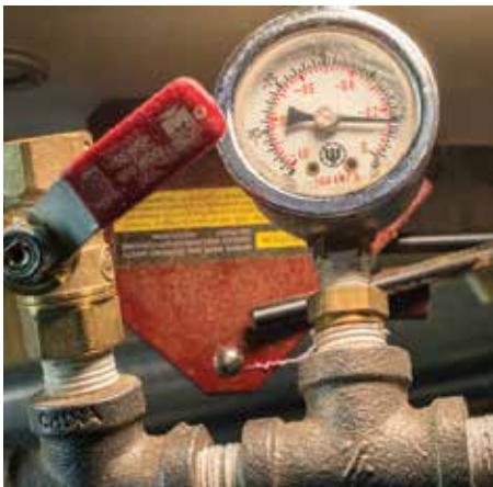
With the larger chuck, the vacuum was 1/7th of the maximum to very safely hold that platter
