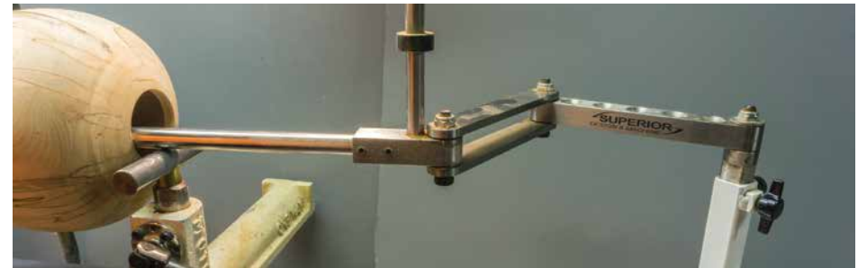
A scissors type design implemented on one of my small lathes. No need for the guide trap by design
