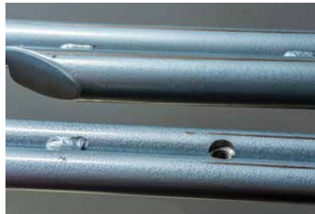
The dampening of both size systems is considerable with the dual welded bars of 5/8in or 1 1/4in
