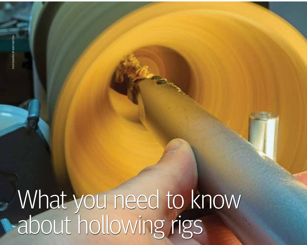
Care must be taken to ensure your bar doesn't slip off your toolrest. Custom hollowing rigs provide stops
