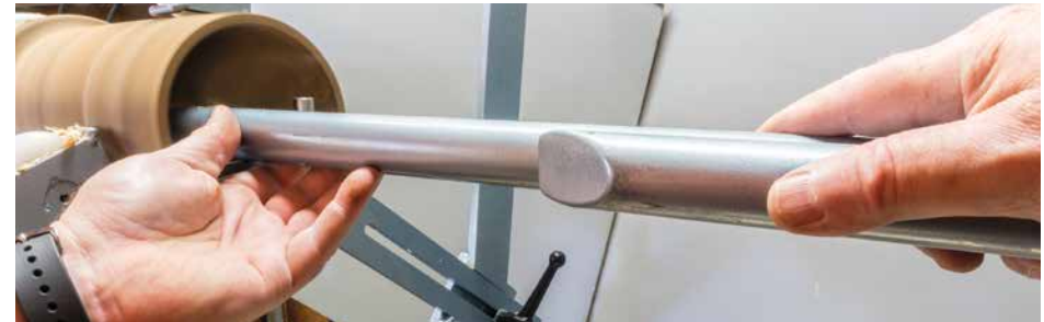
My large welded side by side bar hollowing system. Massive dampening and long over toolrest reach
