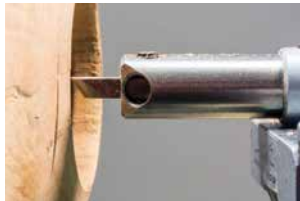
I set my cutter working edge height to be ever so slightly above the centreline of the work
