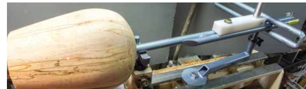
Hollowing systems offer a laser attachment that will help with determining wall thickness as you are cutting
