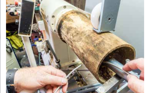
My favourite is the simple coat hanger or welding rod closed to a gap and then compared as slid inside
