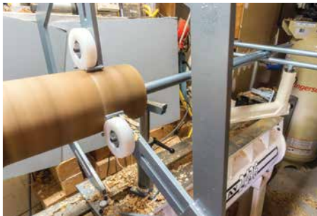
My larger hollowing rig with a 1 1/4in bar can reach 33in over the toolrest
