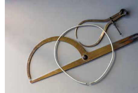
Wall thickness can be measured with any of the standard measuring tools that will reach
