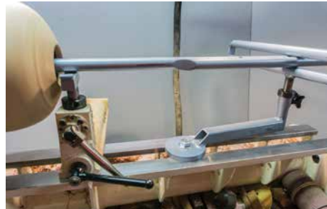
Made for smaller lathes, this hollowing rig is capable of about 9in reach over the toolrest
