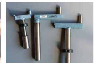
I favour the high strength toolrests with movable pins. Note the rest on the left with adapter sleeve partially slid on
