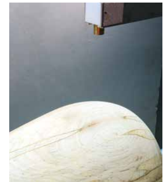
Adjusted to your desired wall thickness, when the laser beam falls off the edge of the turning you are there
