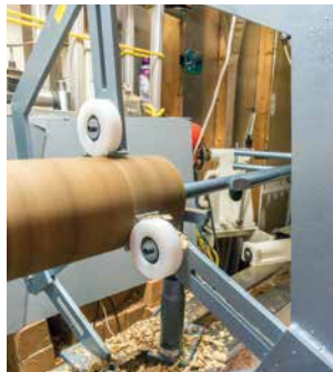
Centre steadies are available in several designs and in sizes appropriate for your work and lathe
