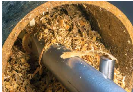
The debris needs to be cleaned periodically to allow for effective cutting. An air hose works well
