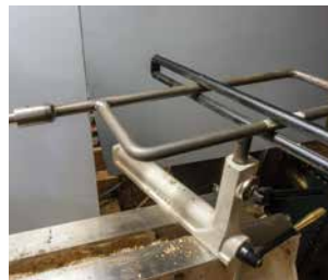
One of the early designs of the captured hollowing bar system. Still working well
