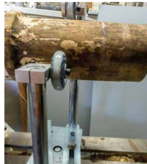
One of the newer centre steady designs whose frame doesn't surround the work
