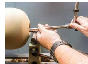
The standard banjo and toolrest will work well provided you work over the toolpost for maximum strength
