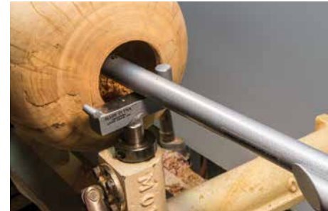
Care must be taken to ensure your bar doesn't slip off your toolrest. Custom hollowing rigs provide stops
