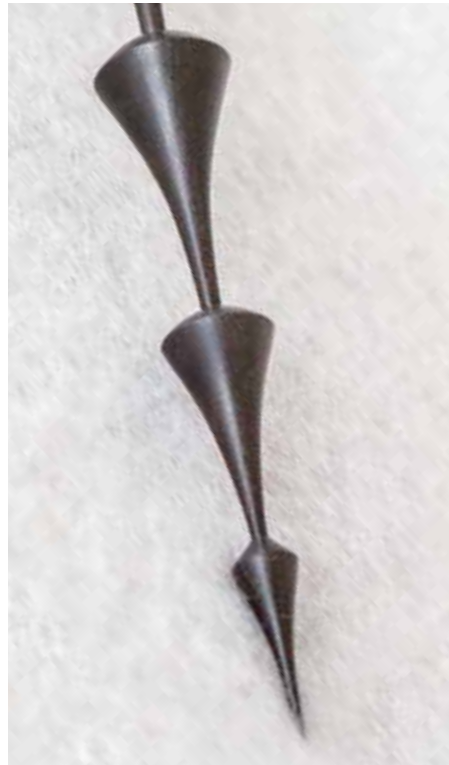
If you intend to turn thin, resembling melting icicles for example, straight grain dense wood is critical
