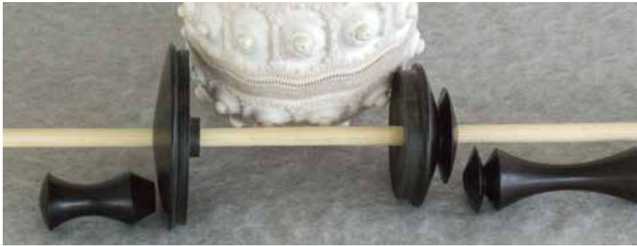
By design, only wood-to-wood glue joints using the bamboo rod to bond all of the blackwood pieces
