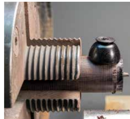
Any sized chuck or collet can be used if you are willing to cut away and waste wood; I try to use mounts that hold near finished size
