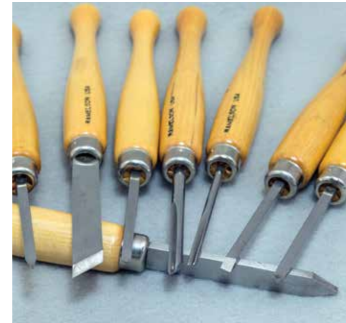
Miniature turning tool sets are available but they require adaptation of most full sized grinding setups
