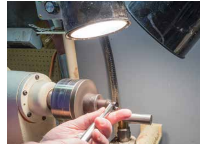
You can never have too much light when turning small or miniatures: goose neck lamps allow for easy positioning
