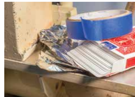
When shimming is required for alignment, playing cards, tape, or a proper amount of folded aluminium foil will work well
