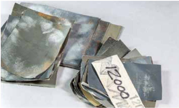
Usually the Micro-Mesh range is sufficient. Cut your Micro-Mesh to fit the work being done and mark the back of smaller pieces
