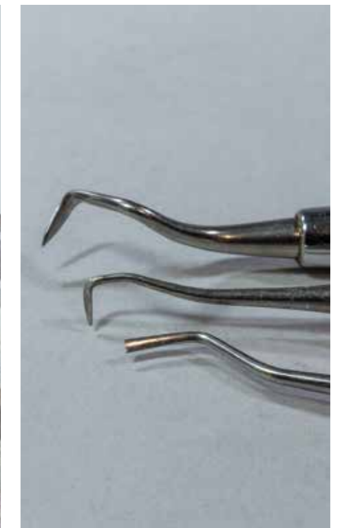
I find that dental picks can be reshaped and ground to suit: they are available new and unused via ebay
