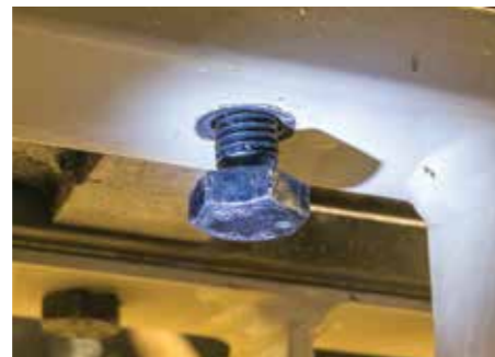
Whether bolted from the top or bottom, nearly all headstock mounting holes have some room for minor alignment adjustment
