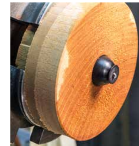
When I jamb chuck miniatures, I cut them snug and then wet the wood to effect the grip. The jamb chuck will swell to grip well
