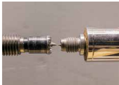
Anything with a sharp point can be used to check headstock to tailstock alignment: take the time to check and adjust for error
