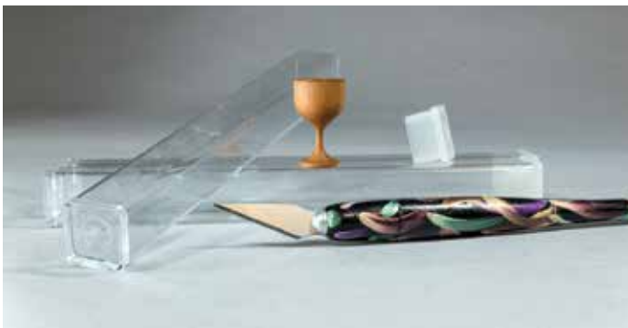
Plastic pen tubes can be cut down with an Xacto knife to create carrying and display cases for turnings that could be easily lost or damaged
