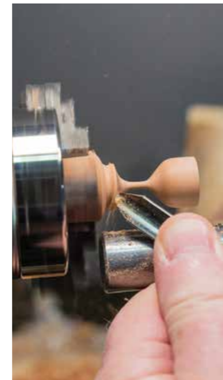
When turning small or miniature work, you can often press full sized tools into service with proper grinds
