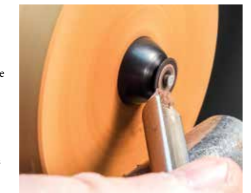
The jamb chuck allows for turning, sanding, and finishing. Easy removal without damage once dry
