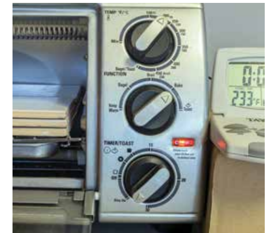
Filling the oven with tiles will add to the thermal mass, shield the clay from the heaters, and moderate temperature variation
