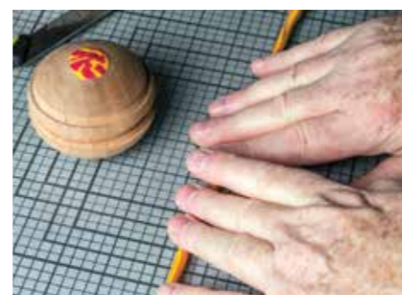
Grooves, relieved areas, cracks or flaws and drilled holes are all candidates for clay insertion
