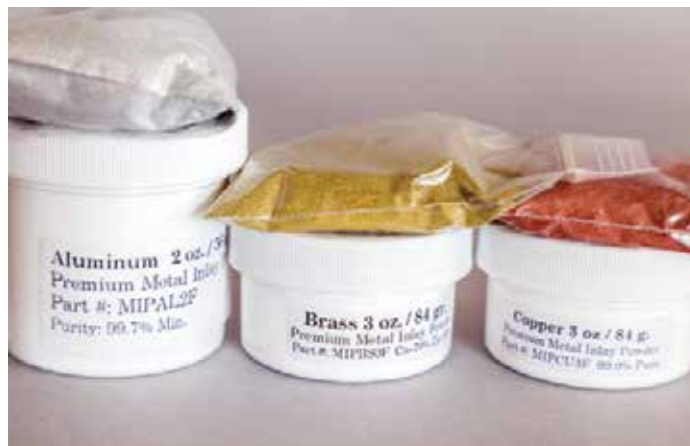
Brass key cuttings will work but commercially available metal powders are cleaner and more uniform in size
