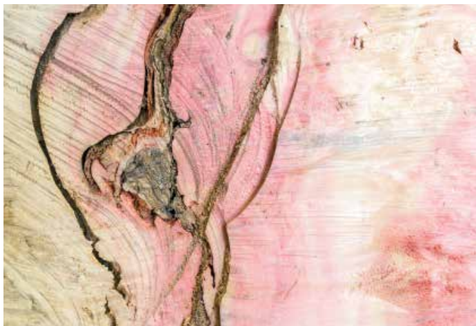
Filling cracks, voids, or other flaws is far easier while in the flat before cutting and turning
