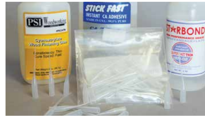
Thin and very thin cyanoacrylate adhesive fastens metals and stone in place, made easier with precision dispensing tips
