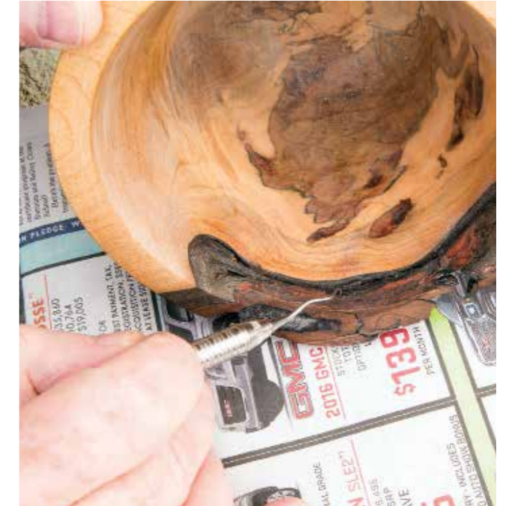
Remove anything that is likely to come loose. A good clean bonding area will ensure longevity
