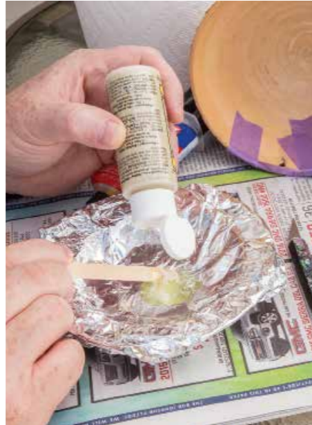
Regular two-part epoxy can be used and coloured with regular artists acrylic paint
