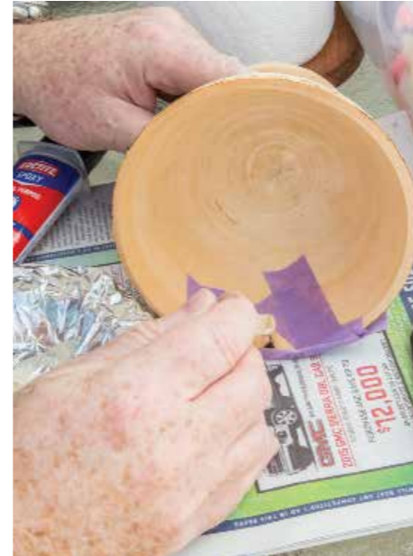
With everything ready, you'll need to mix the epoxy, blend in the colorant and apply within the open time
