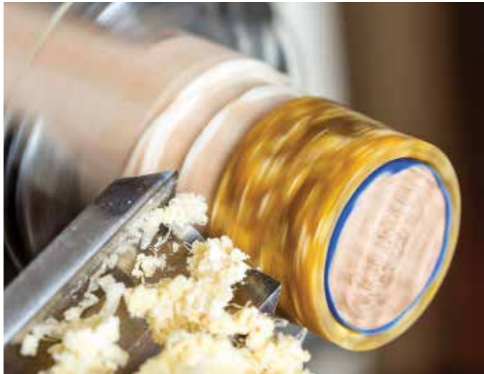
Plastics are far more forgiving when making rings. They have no grain orientation to cause fragility and they turn and polish nicely. I find a roughing gouge works well to thin walls to the desired dimension. You can use any cutting tool with which you are comfortable.
