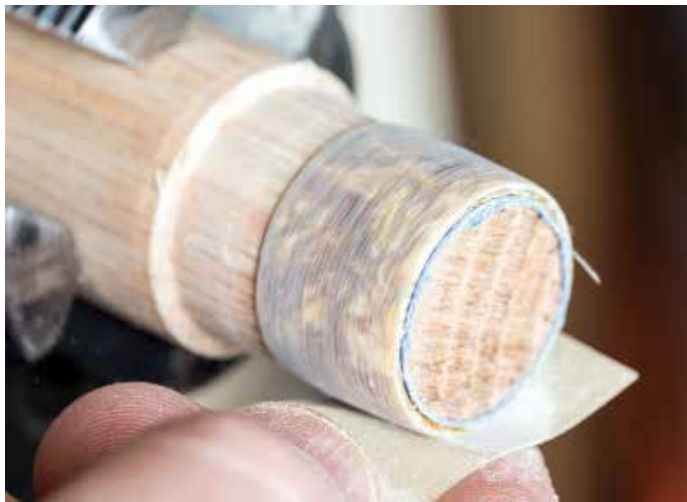
Regardless of your material, turn to just larger than your finished dimension with any shaping needed and then use abrasives to get to the final finish. Nearly all abrasives will work much better when the lathe is run slowly and they are allowed to cut.
