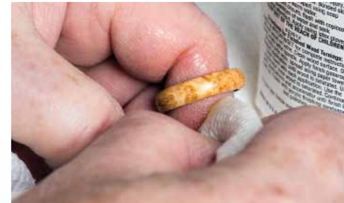
Plastics usually need no finish. For woods, use the finish of your choice to protect it and make the grain pop. I use a wiping oil for a matte finish and a cyanoacrylate adhesive for a gloss finish. If you are new to a cyanoacrylate finish, learn the procedure before you become very attached to your work!
