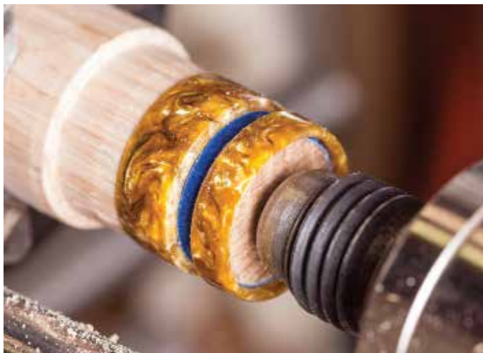
'V' cuts made with a skew chisel make short work of material in this wall thickness. The tail centre is brought up to keep the cut-off section of the ring from getting lost should it have come free. It also aids in supporting the end of the mandrel, although is not really required.
