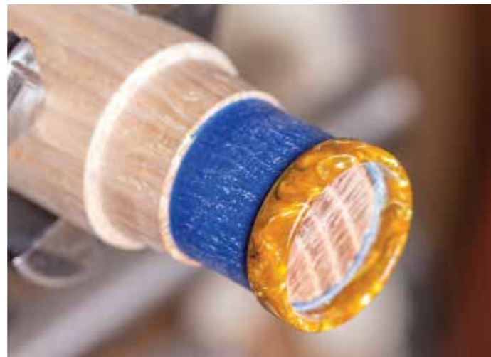
The rings can be positioned on the mandrel so that the cut ends can be sanded through the grits and taken to the desired finish. Sometimes a bit more tape is needed to allow the ring to overhang a bit, giving access to the inner edge.
