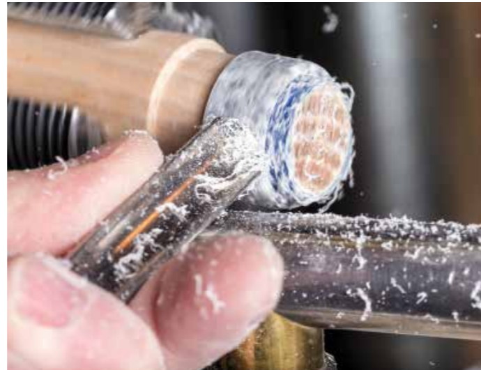
Use a spindle gouge to create a special curvature or features in a ring. In this picture, a thicker, more rounded profile ring is made from Corian. The beauty of a wooden mandrel is that you can cut into it without danger and easily create another when it becomes unusable.
