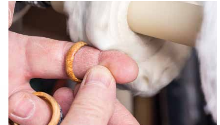
Nearly any material you could use for a ring will benefit from a visit to the buffing wheel. Even raw woods and matte finish woods will show better using a jewellers rouge on a buffing wheel. Run the buff slowly enough to let the rouge and the buff do the work.
