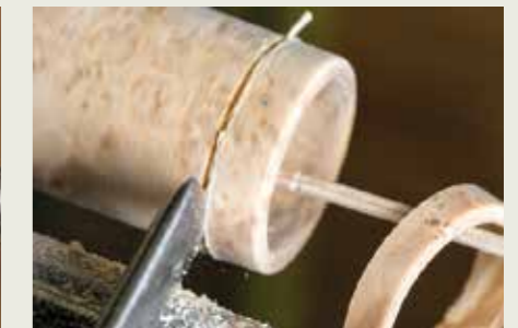
Sand the inner diameter to finish and the outer diameter with the coarser grits. A tooth pick in a drill chuck in the tailstock helps capture the rings as you cut them off at the desired widths. 'V' cuts with a skew chisel work well. Sand the cut ends on the end of the mandrel as before.
