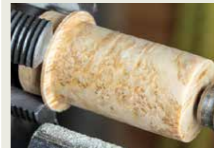
Another method of making rings from square or round stock is to turn it round between centres. Put a tenon on a short length of the material and mount it in a chuck. Turn the outer diameter slightly proud of the desired finished diameter.
