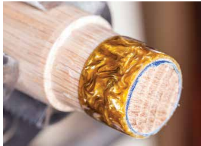
The inner and outer surfaces have now been taken to the final finish and the ring wall thickness is as desired. This blank was too thick for a comfortable width ring, so now is the time to deal with the ring width.
