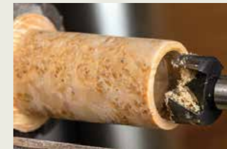
Use the Forstner bit to cut the inner diameter slightly smaller than desired. Work in stages as you move towards the headstock. Drill a small depth, then repeat the process.
