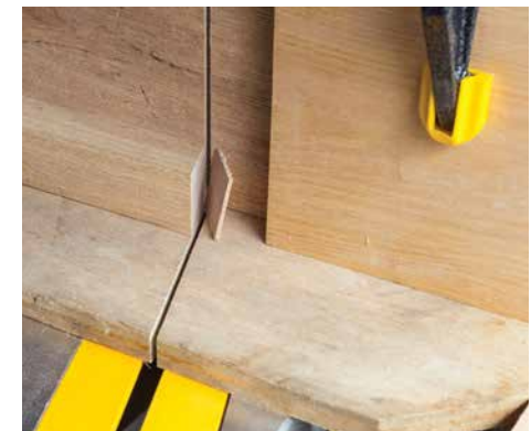
With good stock support, most saws can produce very good quality cuts
