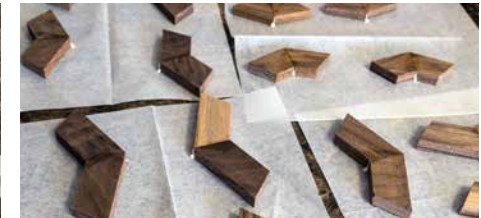
The segments are glued up in pairs and allowed to cure. Then pairs of pairs are glued up
