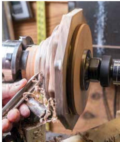
Turning a segmented blank is like other bowl blanks. Use the same tools, sharp tools, light touch, and cut downhill
