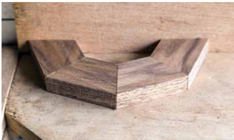
Making your shortest cut length first, take the first four and double check your angle stackup. Alter if needed
