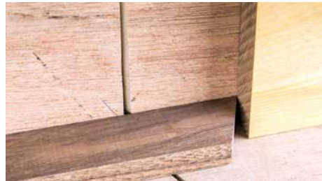
Make the initial angle cut to establish that. Flip the stock 180°, position at the stop and cut the segment
