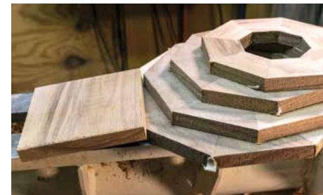
Glue squeeze out and uneven segments need to be sanded prior to blank glue up
