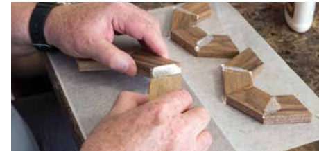
The 'rub joint' is a quick and easy gluing technique. It can be accomplished in moments, with no clamping
