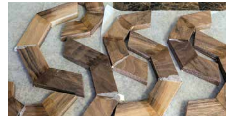
Once you've arrived at halves, any angle error needs to be corrected before full rings are created
