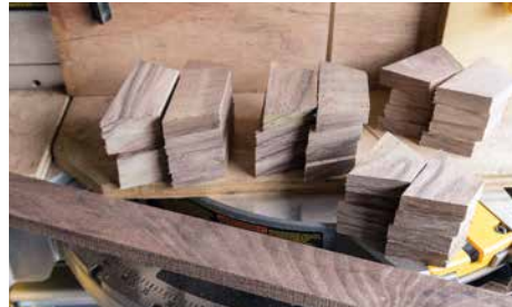
Once things are adjusted, cutting segments is quick work. Cut them all and save extra stock in case of errors later
