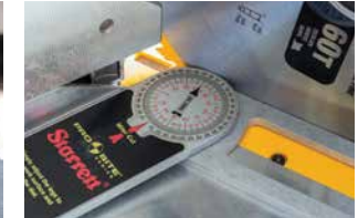
Insufficient resolution or accuracy. A tenth of a degree error times 16 cuts is a 1.6° problem
