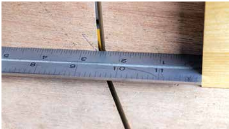
Setting the stop block accurately will help produce your planned results. Not the place for a tape measure
