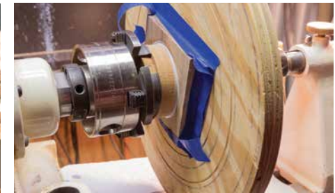
Waste block prepared, the base is glued and clamped in place using a home made centring platen in the tail stock
