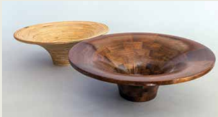
Whether solid wood or plywood, your segmented blank can present you face grain for your cutting
