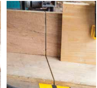
Cutting segments from scrap and checking the error stackup lets you tweak the angle setting until correct
