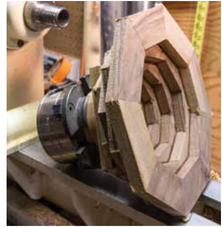
The completed segmented blank ready for turning
