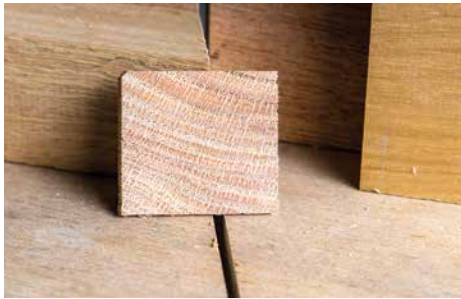
A sharp blade, proper speeds and feeds, and good stock support yields clean high quality cuts
