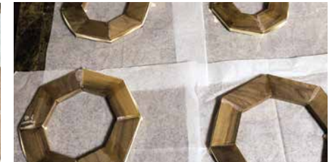
When the two halves mated perfectly, they can be glued together. You may wish to use rubber bands for compression
