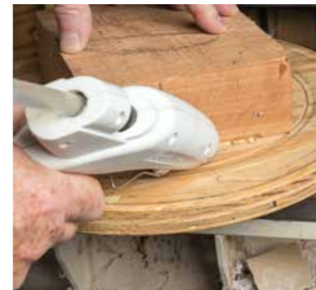
No drill press? Use your lathe. Your stock can be attached to a faceplate with a backer using hot melt adhesive
