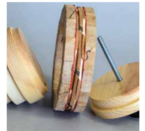
A clever chuck mounted clamp for bracelets Nelson devised and uses with his youth program students
