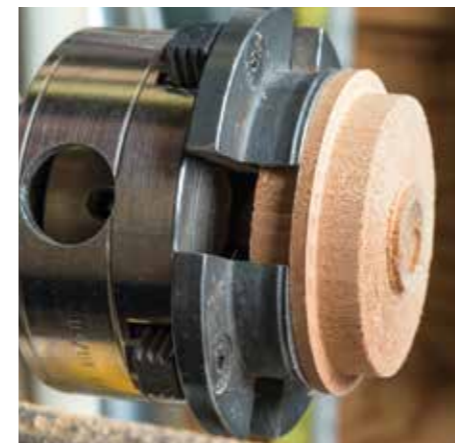
A jamb chuck turned at the moment to fit the occasion. Any scrap works, a shoulder is helpful, and tape adapts within reason
