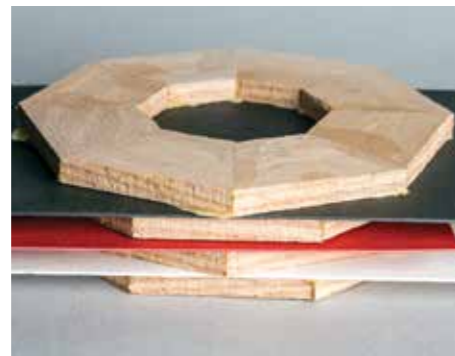
This stack of segmented rings illustrates the strength improvement of staggered seams
