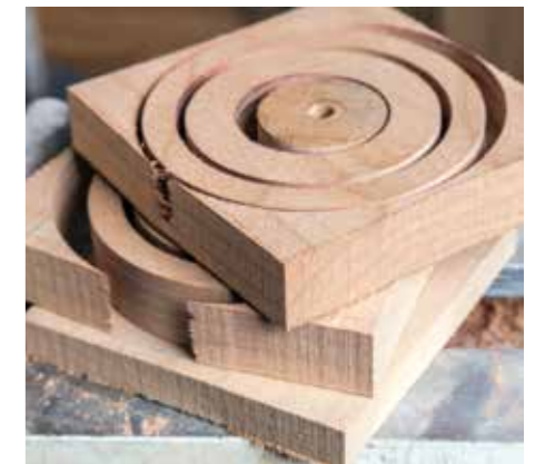
A trip to the band saw to separate the blanks at the desired blank widths in multiples at a time
