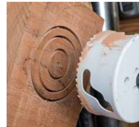
A parting tool or hole saws can be used to create multiple sized bracelet blanks, reducing waste
