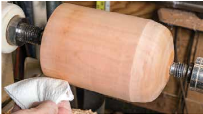
With the lathe running slowly, dependant on the work piece size, apply the accelerator to the surface entirely. You may not see wetting
