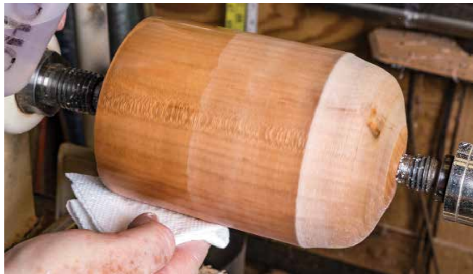
It is good practice to clean the final surface prior to finish application. Here a practice piece is wiped down with denatured alcohol
