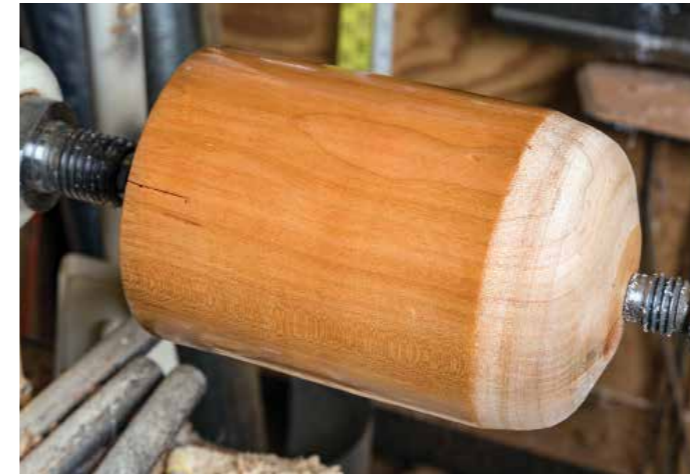
Continue to build to the desired finish. Use the same sequence of one accelerator application followed by three applications of Ca
