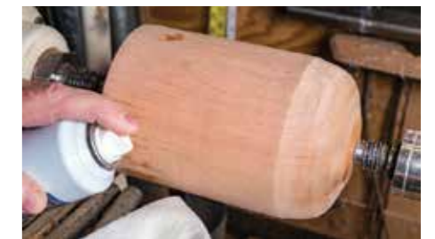
With your alcohol wipe flashing off, spray accelerator on to your folded paper towel. A wet coating but not running or dripping
