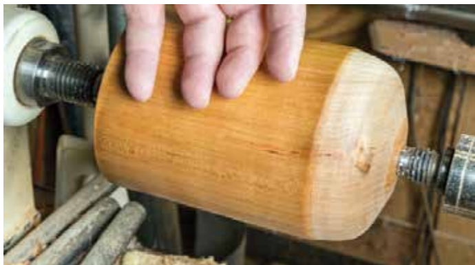
Properly applied, the Ca will cure immediately. If you feel the need to check, use the back of the fingers with a light touch with lathe off
