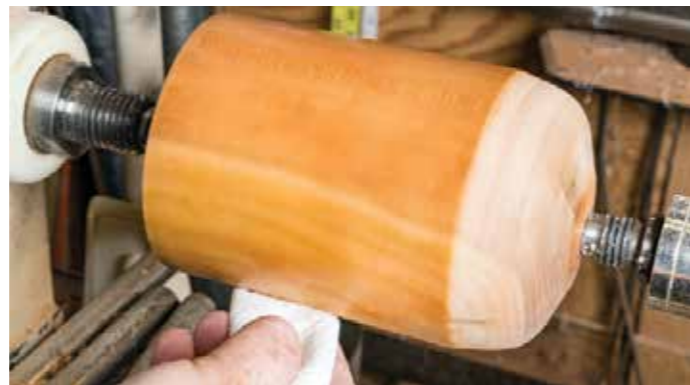
Repeat the Ca application process the same way ensuring complete coverage until three Ca applications are complete
