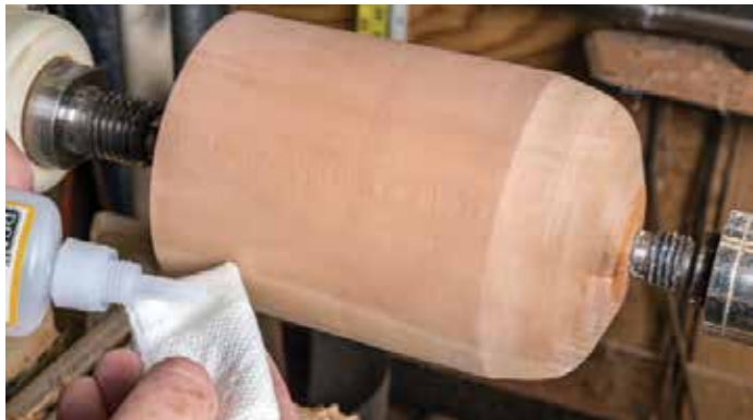
Apply the thin Ca adhesive towards one end of the folded paper towel. Apply enough to make a good wet spot but not sopping wet
