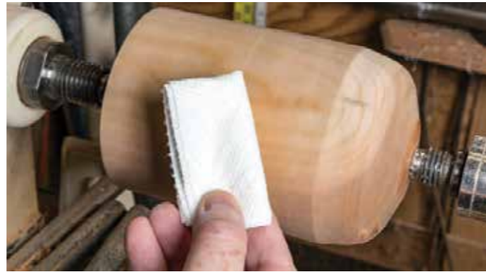
Fold a clean paper towel segment thick enough to protect your fingers from the wicking of the Ca and from the heat generated
