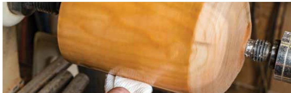
Repeat the accelerator application being sure that the application towel has dried prior to applying to the work. Apply three more Ca coats
