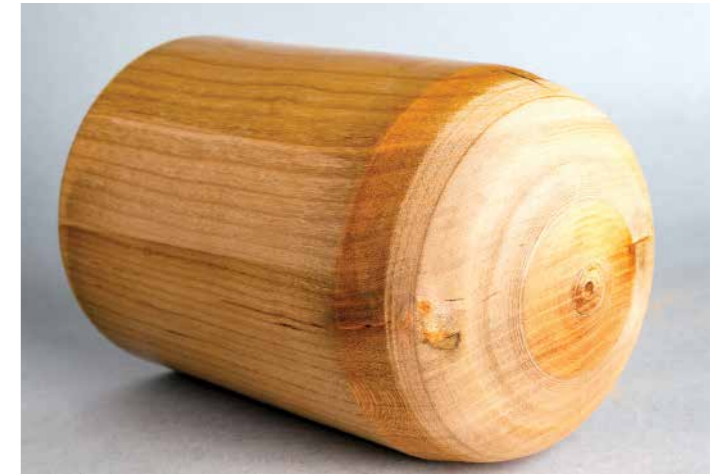
The practice piece with only six coats of Ca applied to the flat cylinder surface. No leveling, sanding, or buffing yet. Imagine 20 coats
