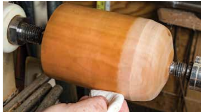
With the lathe still running, wipe on the Ca adhesive flowing from one end to the other. You will see the wetting occur
