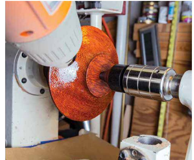
A heat gun set to warm kept well away from the turning can lower the viscosity for penetration as well as accelerate the curing
