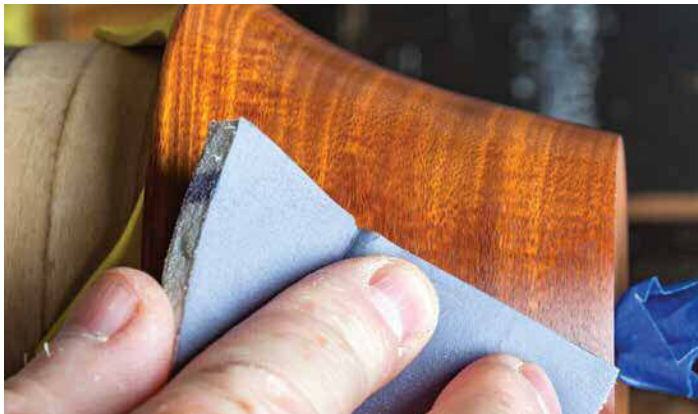
Once at the final coat, 1 or a number of them, a final sanding through the Micromesh will smooth and shine to a gloss if desired
