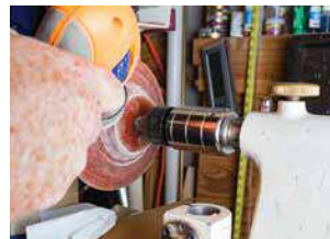
Sanding between coats with 330 to provide tooth for the next coat. If you don't get white dust, you haven't let it cure enough
