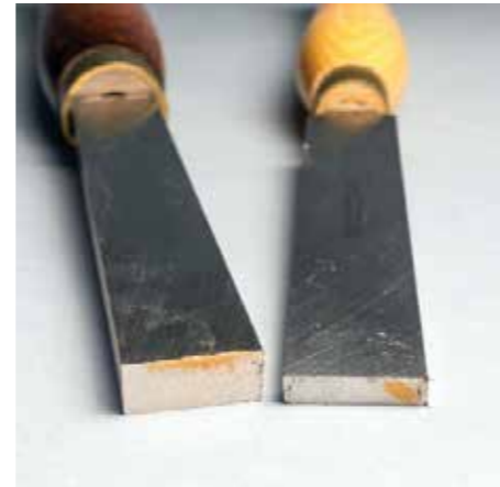
Given a choice, always reach for the more massive tool if it can possibly fit your application
