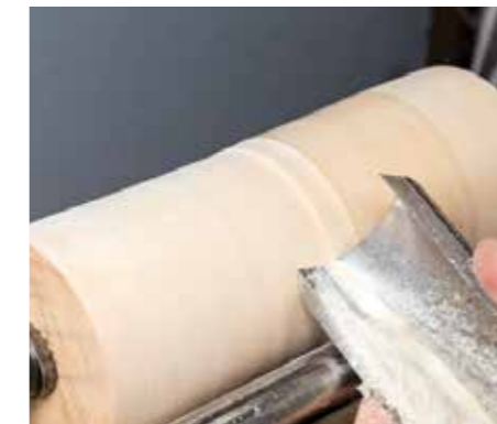
Controlled engagement is the key to nice ribbons of wood being cut away
