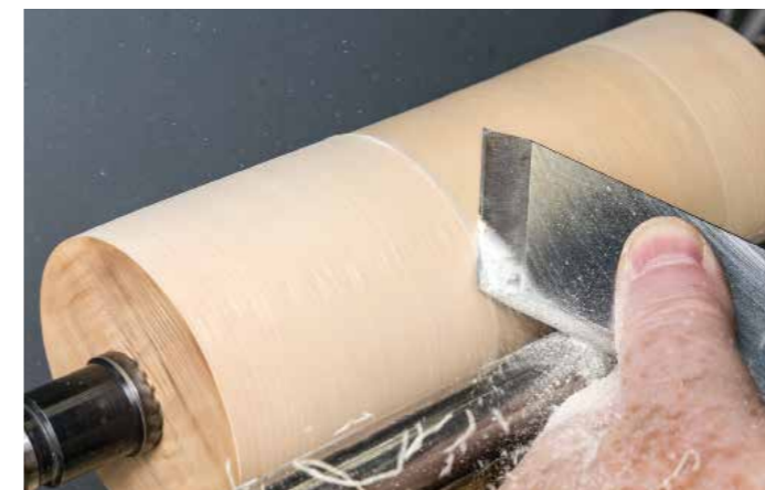
With the sweet spot between 25 and 50% of the edge, the bigger the tool, the bigger the sweet spot
