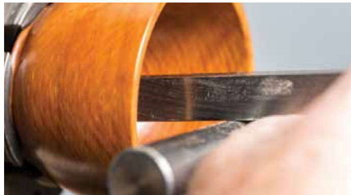
Keeping your reach within reason, a sturdier tool will not flex away from your cut or scrape
