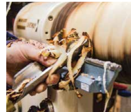
For the most part, a large spindle roughing gouge is the correct tool but be cautious of too much 'edge'
