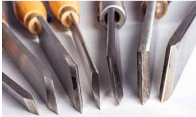
My workhorses. All rectangular shafts except one oval for fitting into very thin openings
