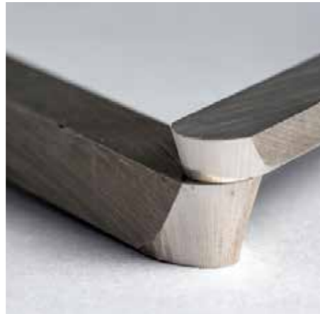
The same scraper face, but two very different tools. The greater mass tool will better dampen vibration
