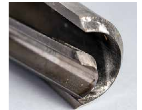
There are occasions when the smaller spindle roughing gouge is in order. Less edge in the mix
