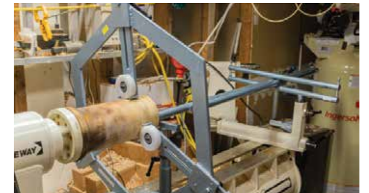
The huge mechanical advantage lies in the long, massive bar that is captured as well
