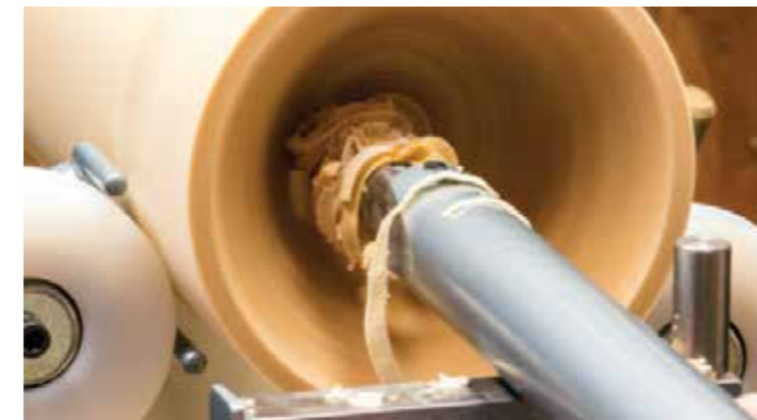
Hollowing rigs make great use of mechanical advantage. It uses support as close as can be done
