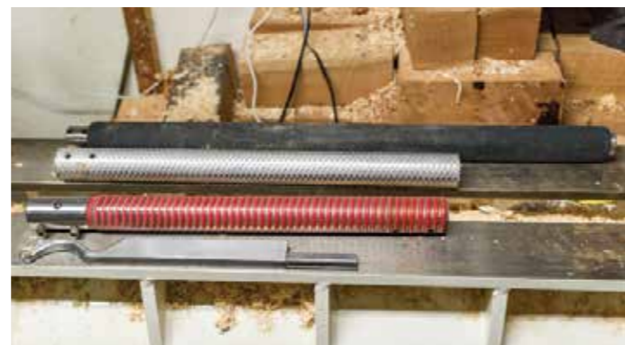
RIGHT: Un-handled tools give you the luxury of selecting the handle length and mass most appropriate
