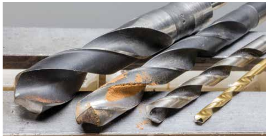
Start small and work your way up to the final size. The quality of the final hole will benefit from the process
