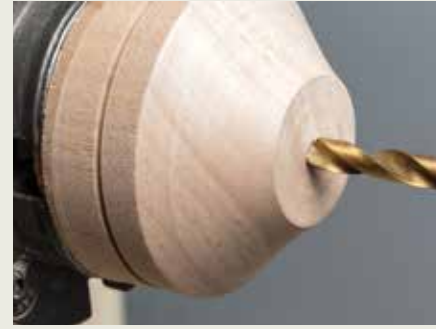
The advantage of a starting location can't be stressed enough. No wander, no drift, easy starting with a place to begin
