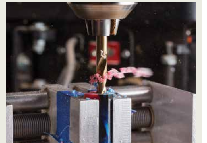
Breaking the chip, easier in a drill press, is good practice to keep the chip strings short and safe
