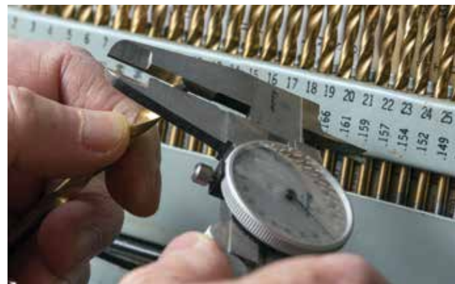
If size is important, measure! You measure a drill diameter across the edges that do the cutting
