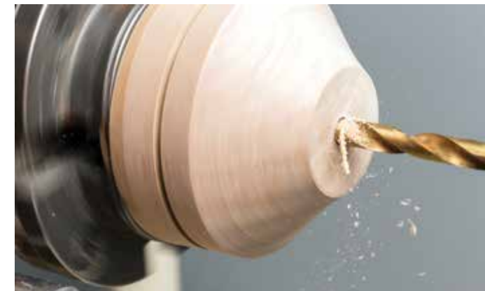
Proper speeds and feeds will drill efficiently, without overheating, and will eject debris effectively
