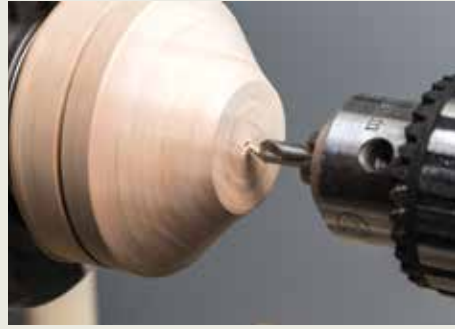
For speed and convenience, I keep a machinist's centre drill chucked up in an inexpensive chuck with its own taper
