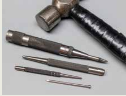
Whether a punch, centre drill or any implement to create a starting 'hole', give yourself the advantage of a starting location
