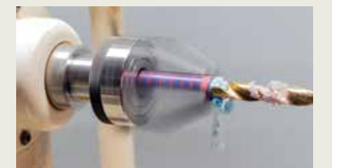
Don't be afraid to practise. Take scraps and drill holes. Try long lengths with thin walls and then check for uniformity
