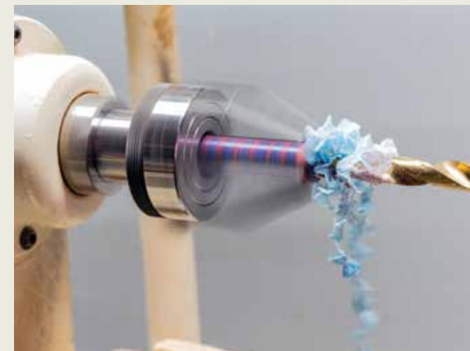
The already cut debris exiting quickly and continuously lets the cutters have a clean area to work
