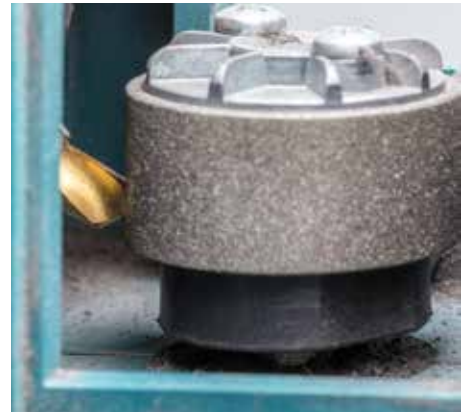
My drill sharpener accurately positions and presents the bit to the diamond wheel when it is running. Safety cover removed for visibility
