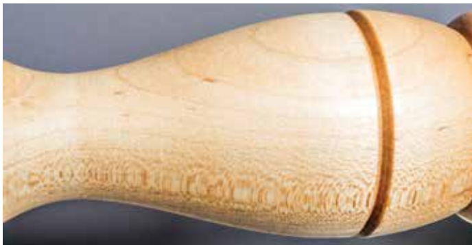
Remember poor turning and poor prep show through on any clear finish. Spend the time in prep to avoid this
